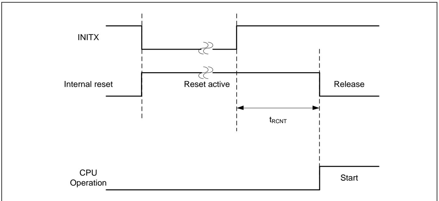
**Operation example of return from low power consumption mode (by internal resource reset\*)**
