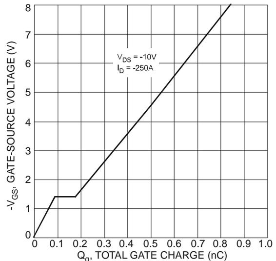
Fig. 12 Gate-Charge Characteristics
