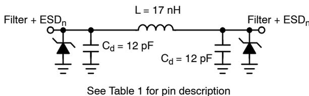
Figure 1. Electrical Schematic
