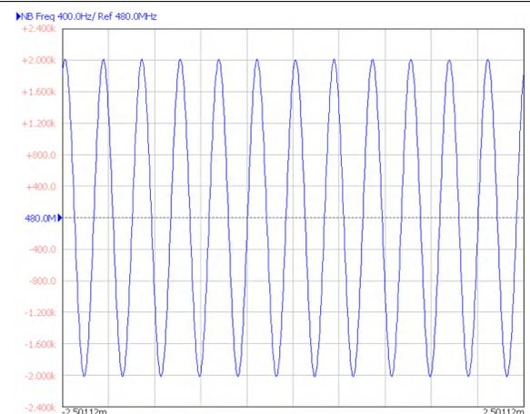
Reference clock is a FM modulated signal with  $f_{MOD} = 2.4$  kHz
