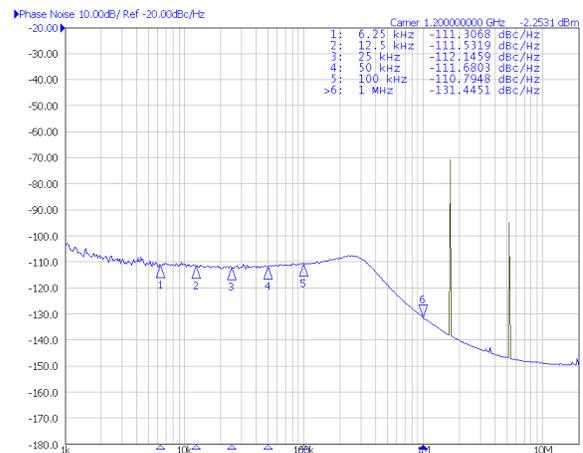
OSCin = 19.44 MHz  $f_{OUT} = 1200$  MHz Synthesizer mode
