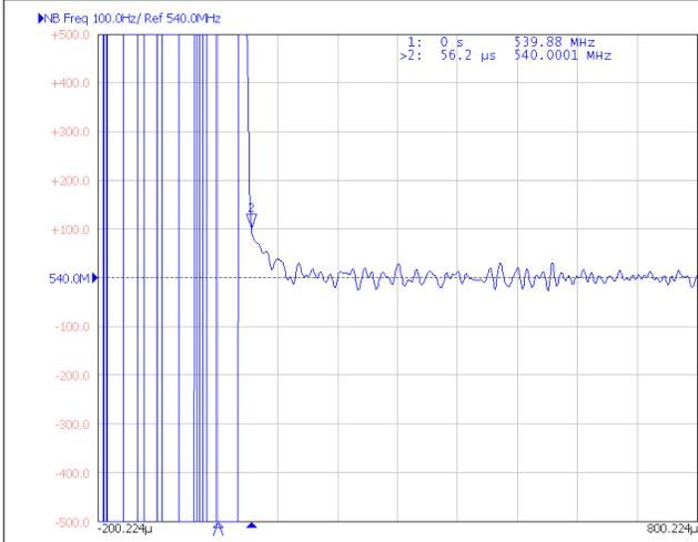
**Figure 8-32. External VCO to Internal VCO Switching Time**
