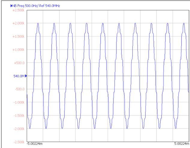
Figure 8-34. Simulated FM Modulation (10 Times Over-Sampling)
