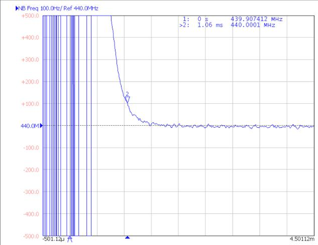
**Figure 8-33. Internal VCO to External VCO Switching Time**
