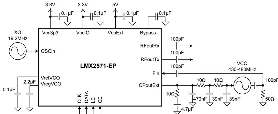
**Figure 8-28. Typical Synthesizer/PLL Duplex Mode Application Schematic**
