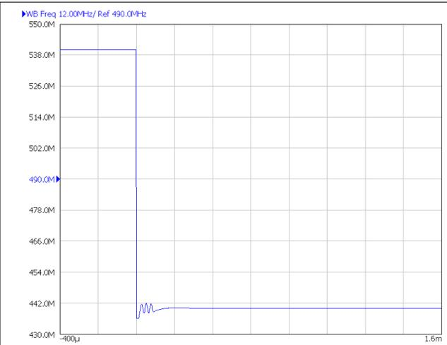
**Figure 8-31. Internal VCO to External VCO Switching**
