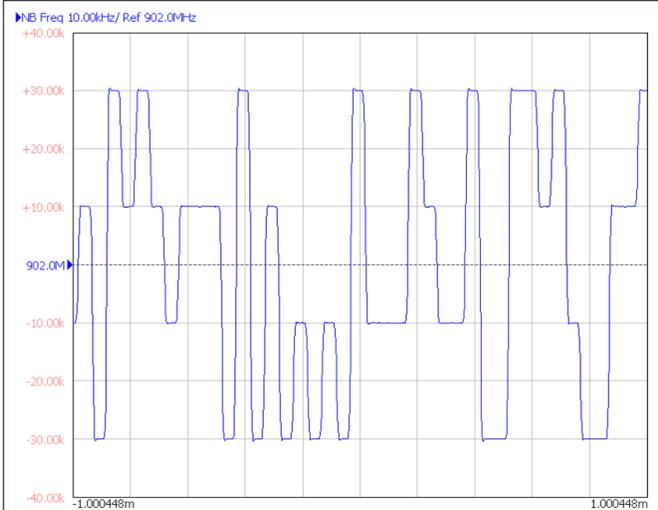
**Figure 8-20. 4FSK Modulation**
