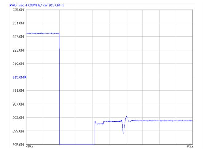
**Figure 8-17. F2 (RX) to F1 (TX) Switching**
