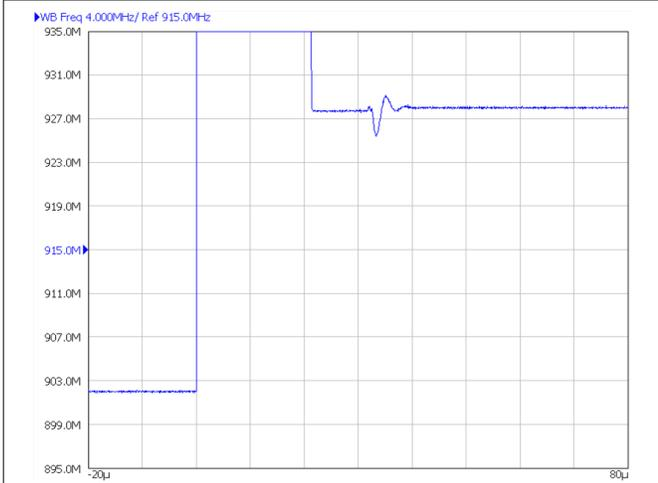
**Figure 8-16. F1 (TX) to F2 (RX) Switching**
