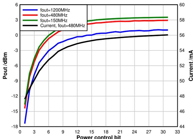
Figure 8-11. Configurable RF Output Power
