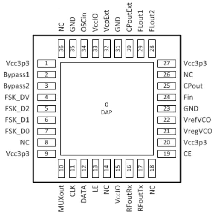
Figure 5-1. RHH Package 36-Pin VQFN Top View
