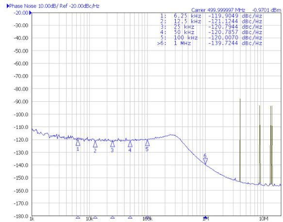
OSCin = 19.44 MHz  $f_{OUT} = 500$  MHz Synthesizer mode
