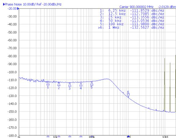
OSCin = 19.44 MHz  $f_{OUT} = 900$  MHz Synthesizer mode
