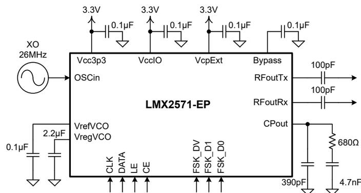
**Figure 8-12. Typical Synthesizer Duplex Mode Application Schematic**
