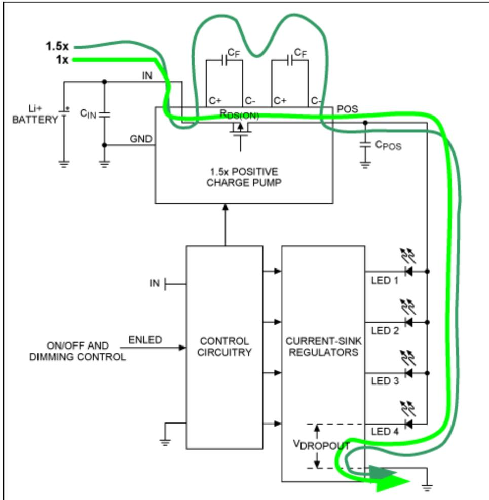
Figure 1. In 1x mode, the positive charge pump uses an internal switch to bypass  $V_{IN}$  to the WLEDs' anodes.
