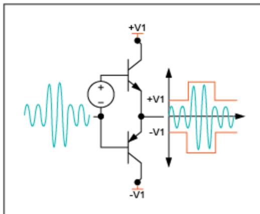
*Figure 7. A Class H audio amp reduces dissipation across the output devices connected to that supply. This allows the amp to operate with an optimized Class AB efficiency, regardless of output power level.*
