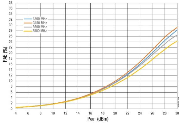
Figure 3. PAE vs Output Power (CW) Across Frequency
