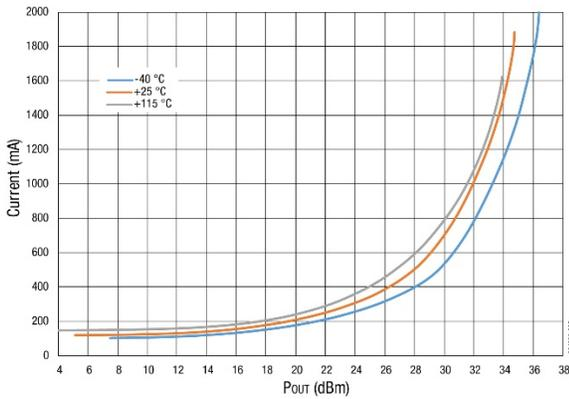
Figure 5. Iop vs Pout Across Temperature @ 3450 MHz, 5 V
