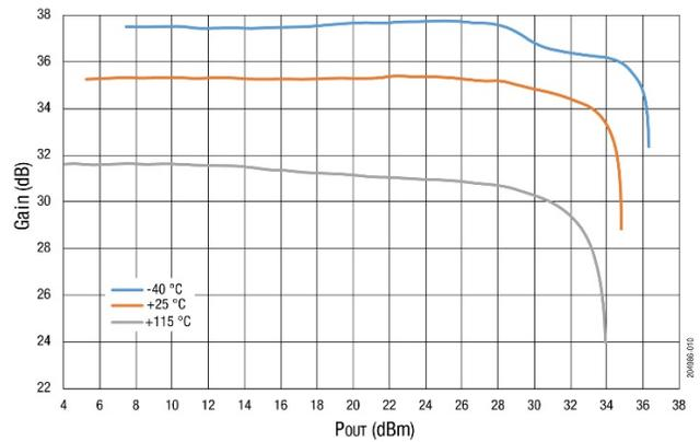
**Figure 10. Gain vs Pout Across Temperature**
