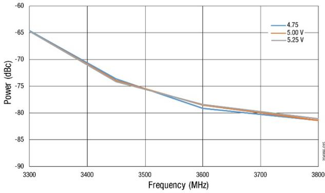
**Figure 15. 3rd Harmonic vs Frequency Across Voltage (P<sub>OUT</sub> = +28 dBm, CW)**
