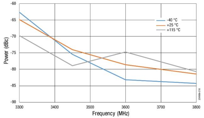
**Figure 16. 3rd Harmonic vs Frequency Across Temperature (P<sub>OUT</sub> = +28 dBm, CW)**
