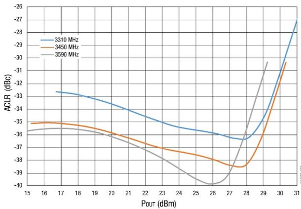
Figure 7. ACLR (1x20 MHz) vs Pout Across Frequency
