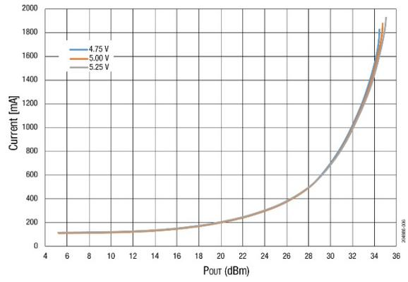
Figure 6. Iop vs Pout Across Vcc @ 3450 MHz, 25 °C
