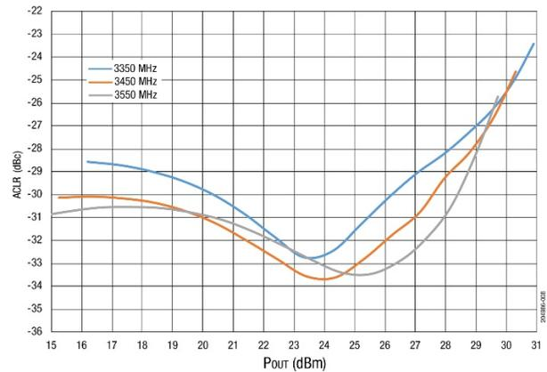
Figure 8. ACLR (5x20MHz) vs Pout Across Frequency
