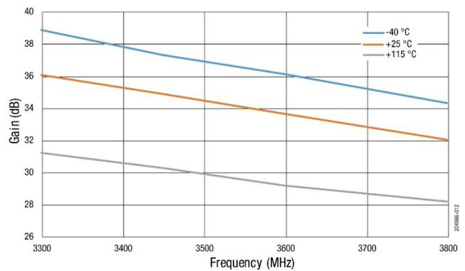
**Figure 12. Gain @ +28 dBm vs Frequency Across Temperature**
