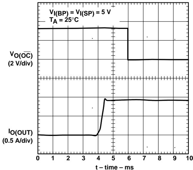
Figure 14.  $\overline{\text{OC}}$  Response (SP Switch), Device Enabled Into Short
