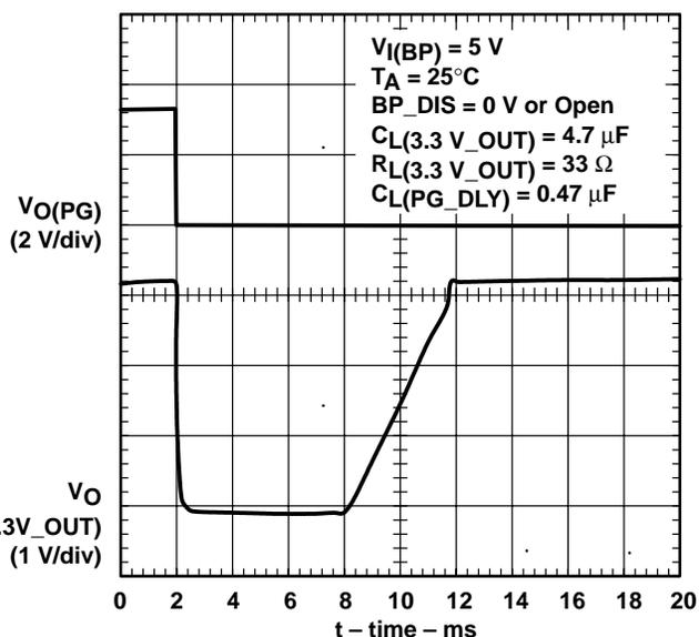
Figure 16. SP to BP Automatic Switchover Enabled
