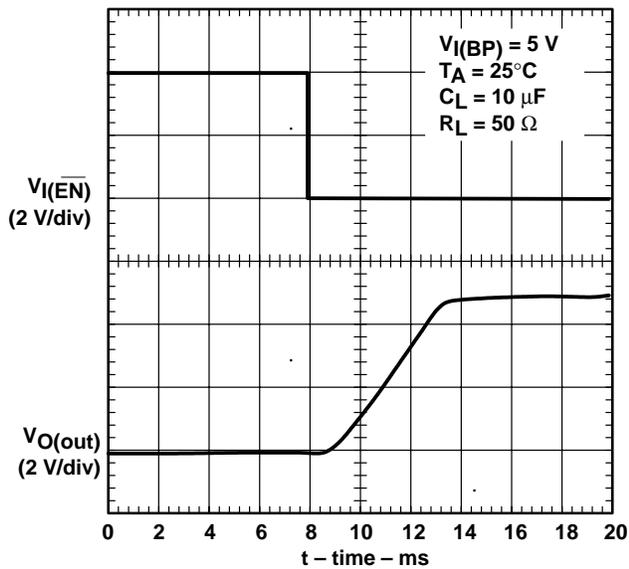
Figure 3. Turnon Delay and Rise Time (BP Switch)
