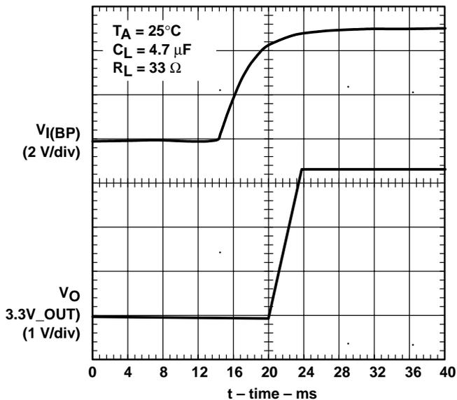
Figure 7. Turnon Delay and Rise Time (3.3V\_OUT)
