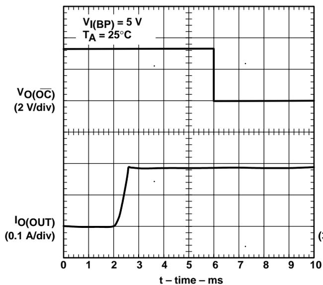
Figure 15.  $\overline{\text{OC}}$  Response (BP Switch), Device Enabled Into Short
