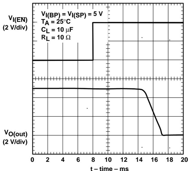
Figure 6. Turnoff Delay and Fall Time (SP Switch)
