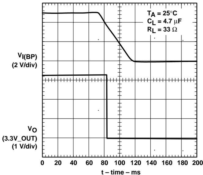
Figure 8. Turnoff Delay and Fall Time (3.3V\_OUT)
