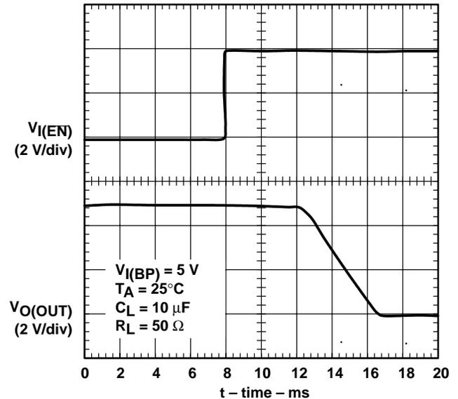
Figure 4. Turnoff Delay and Fall Time (BP Switch)
