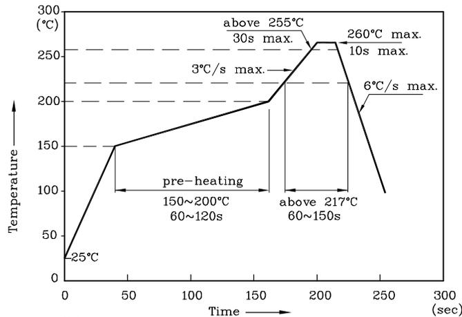
1. All temperatures refer to the center of the package, measured on the package body surface facing up during reflow.
