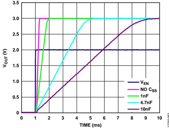
Figure 62. Typical Soft Start Behavior, Different  $C_{SS}$  Values
