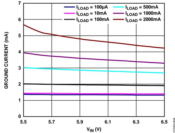
Figure 9. Ground Current vs. Input Voltage ( $V_{IN}$ )
