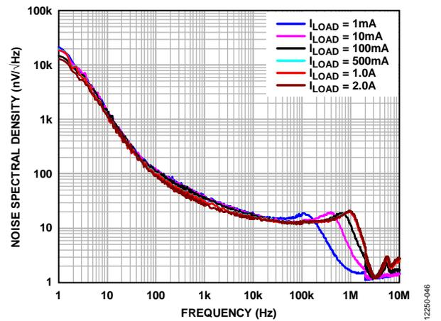
Figure 45. Output Noise Spectral Density,  $V_{OUT} = 5 V$
