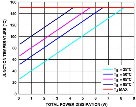
Figure 67. LFCSP Power Dissipation for Various Board Temperatures
