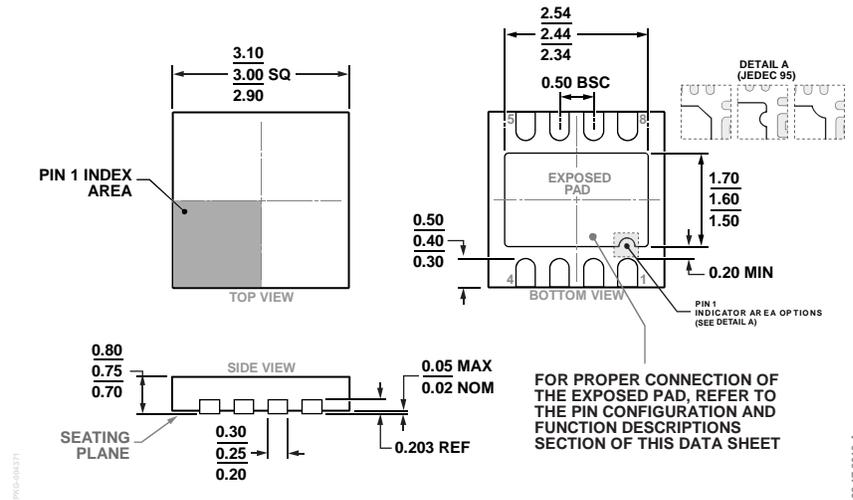
Figure 71. 8-Lead Lead Frame Chip Scale Package [LFCSP]
