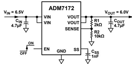
Figure 56. Typical Adjustable Output Voltage Application Schematic
