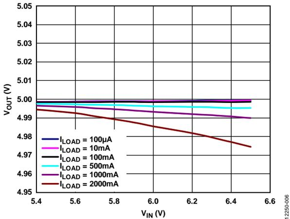
Figure 6. Output Voltage ( $V_{OUT}$ ) vs. Input Voltage ( $V_{IN}$ )
