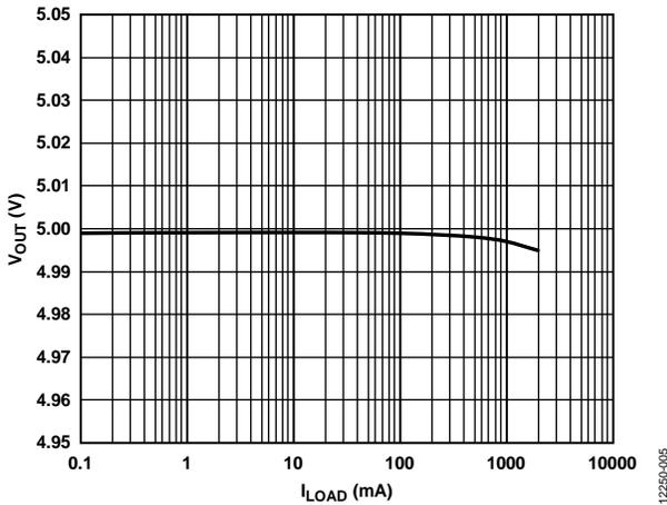
Figure 5. Output Voltage ( $V_{OUT}$ ) vs. Load Current ( $I_{LOAD}$ )
