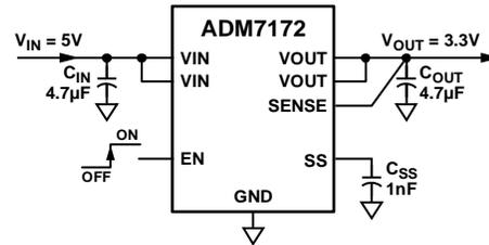
Figure 1. ADM7172 with Fixed Output Voltage, 3.3 V
