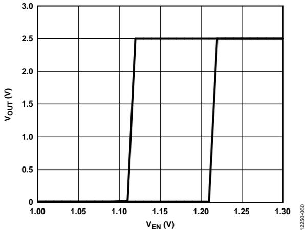
Figure 59. Typical VOUT Response to EN Pin Operation
