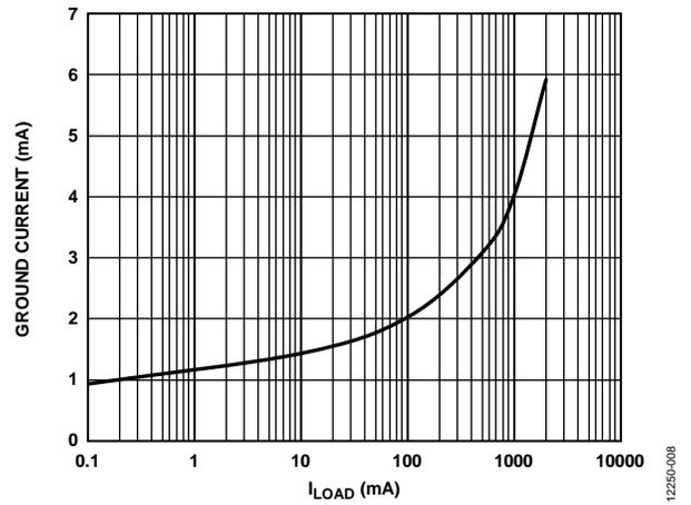
Figure 8. Ground Current vs. Load Current ( $I_{LOAD}$ )
