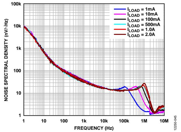
Figure 44. Output Noise Spectral Density,  $V_{OUT} = 3 V$
