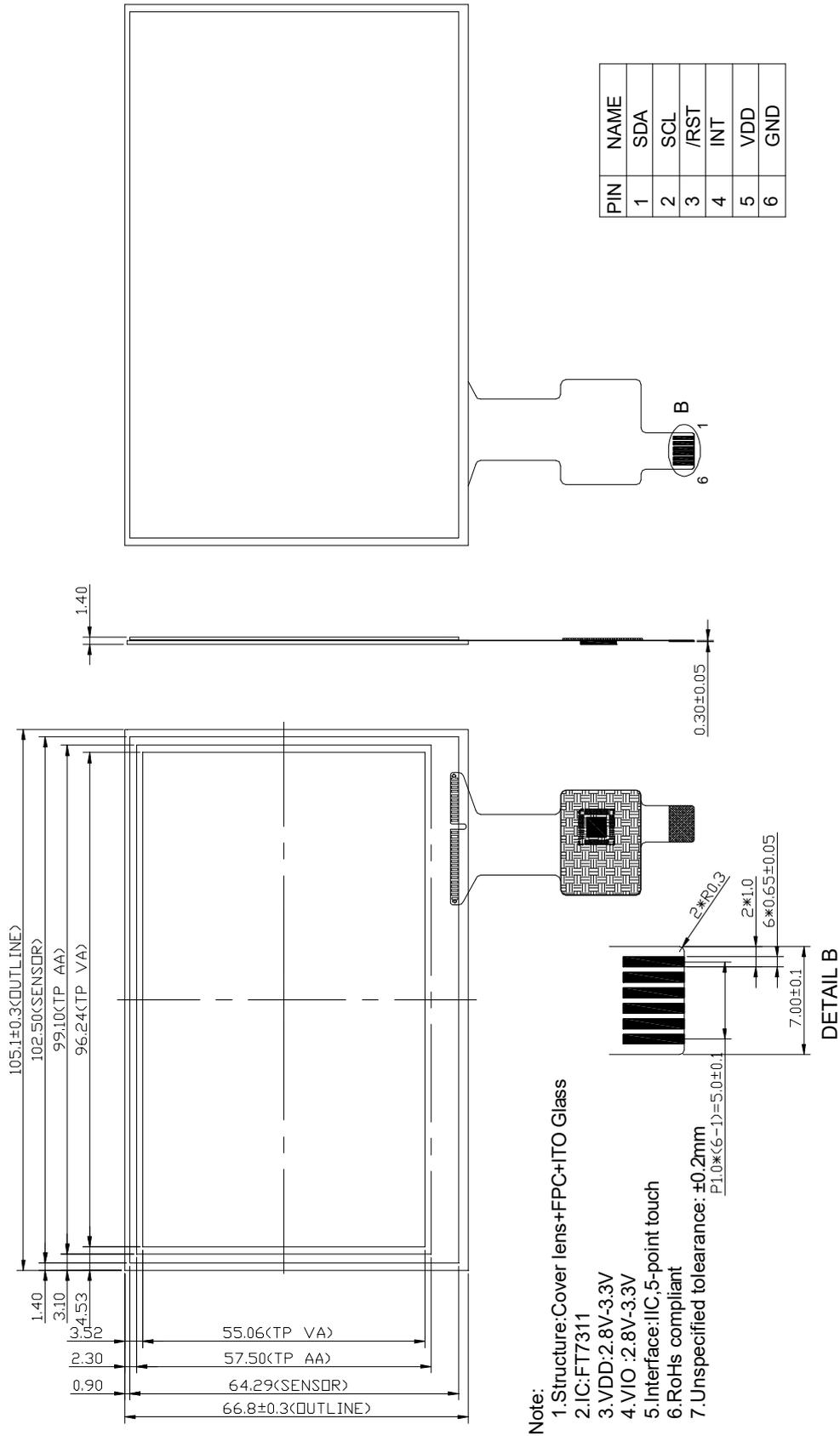
Recommended connector: Hirose FH12-6S-1SH(55) or compatible
