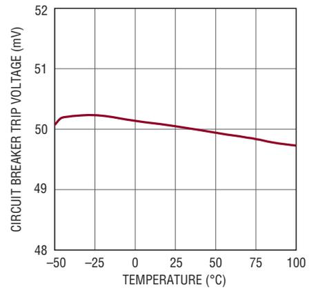
**Active Current Limit Sense Voltage vs Temperature**
