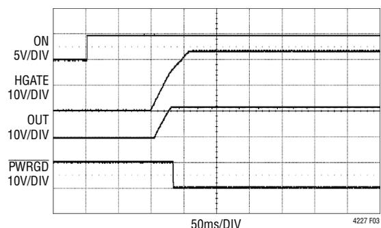
Figure 3. LTC4227-1/LTC4227-2 Hot Swap Controller Power-Up Sequence
