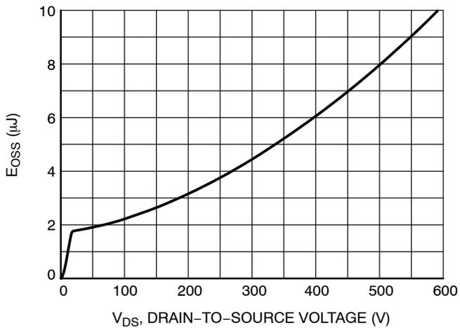
**Figure 11.  $E_{OSS}$  vs. Drain to Source Voltage**
