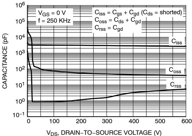
Figure 5. Capacitance Characteristics
