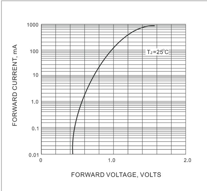
FIG. 1-TYPICAL FORWARD CHARACTERISTIC
