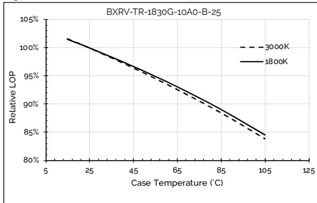
Figure 10: Relative Flux vs. Case Temperature
