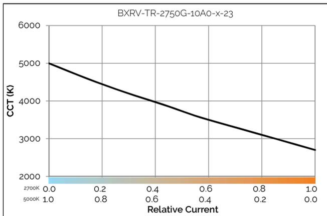
Figure 14: CCT vs. Relative Current, Tc=85C
