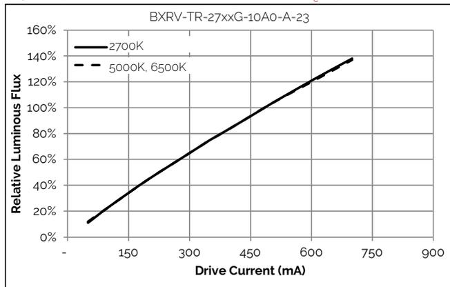
Figure 4: Relative Flux vs. Drive Current,  $T_c=25^\circ\text{C}$
