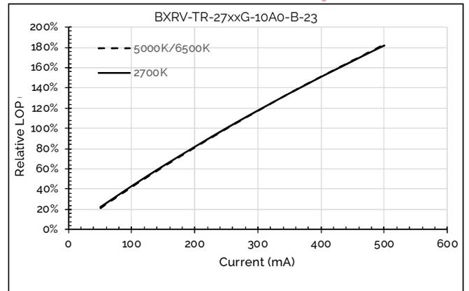
Figure 5: Relative Flux vs. Drive Current,  $T_c=25^\circ\text{C}$
