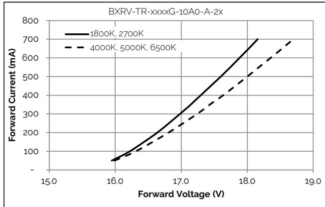
Figure 2: Forward Voltage vs. Forward Current,  $T_c=25^\circ\text{C}$
