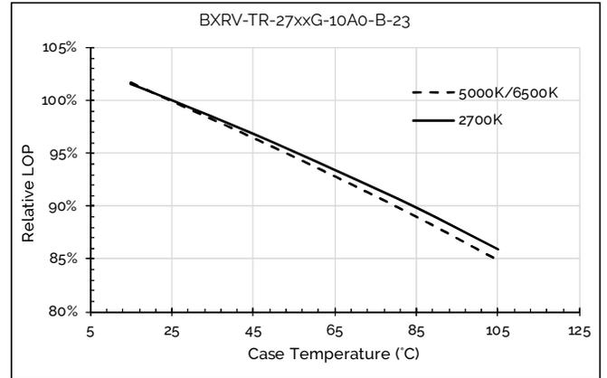
Figure 9: Relative Flux vs. Case Temperature
