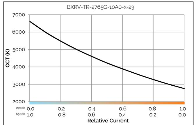
Figure 15: CCT vs. Relative Current, Tc=85C
