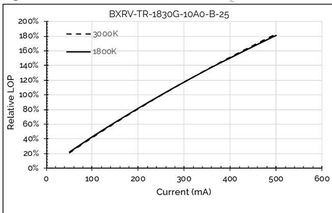
Figure 6: Relative Flux vs. Drive Current,  $T_c=25^\circ\text{C}$
