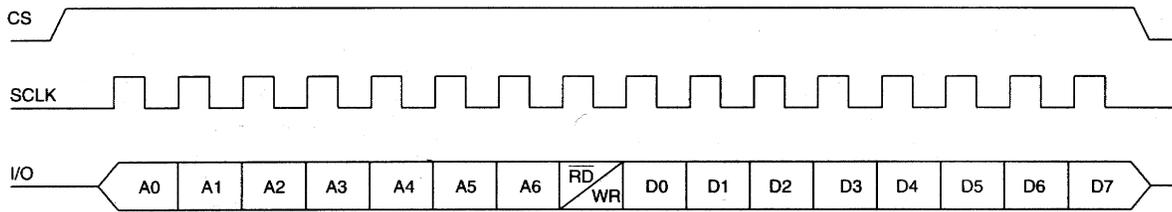
**MULTIPLE-BYTE BURST TRANSFER Figure 8**
