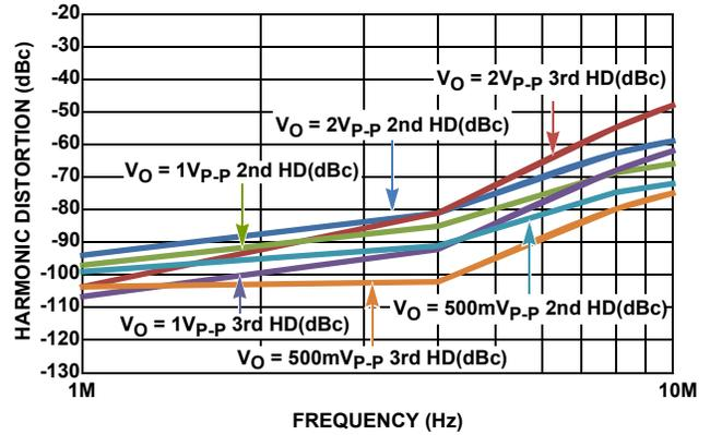
FIGURE 11. INVERTING HD2 AND HD3 vs OUTPUT  $V_{p-p}$
