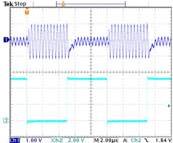
FIGURE 25. INVERTING TURN ON AND TURN OFF DELAY
