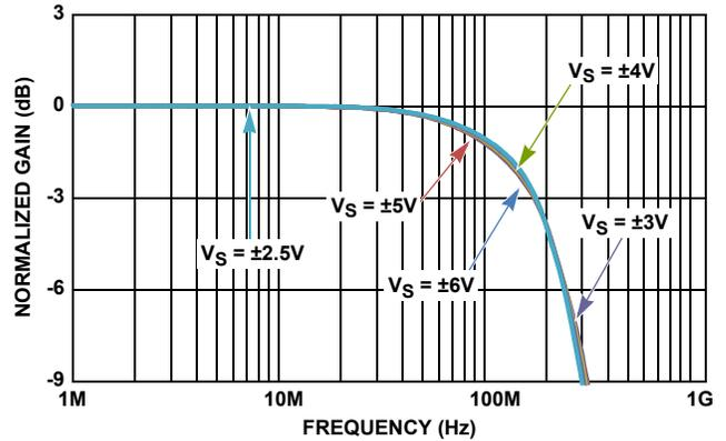
FIGURE 27. INVERTING SMALL SIGNAL RESPONSE VS SUPPLY VOLTAGE
