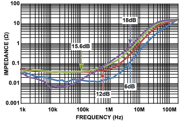
FIGURE 23. CLOSED LOOP OUTPUT IMPEDANCE vs GAIN
