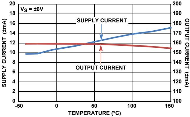
FIGURE 22. SUPPLY CURRENT AND OUTPUT CURRENT OVER-TEMPERATURE
