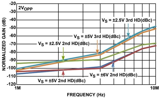
FIGURE 28. NON-INVERTING HD2 AND HD3 vs SUPPLY VOLTAGE
