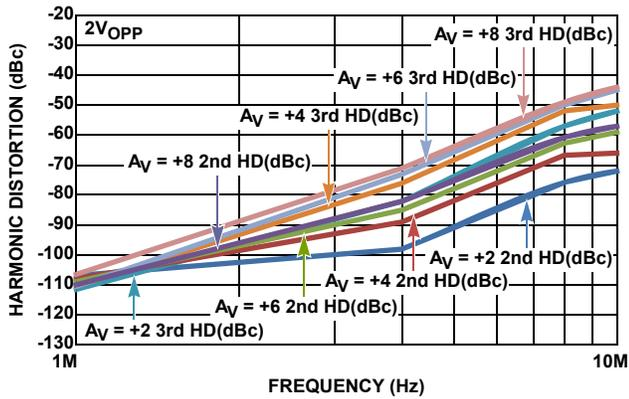
FIGURE 8. NON-INVERTING HD2 AND HD3 vs GAIN
