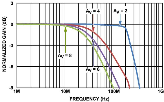
FIGURE 2. NON-INVERTING SMALL SIGNAL FREQUENCY RESPONSE vs GAIN
