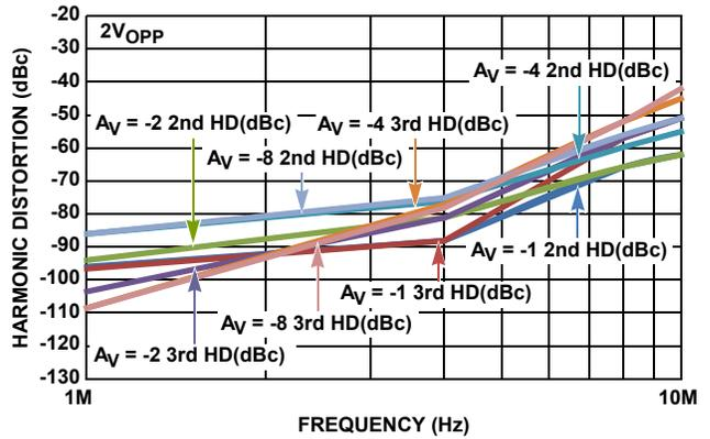
FIGURE 9. INVERTING HD2 AND HD3 vs GAIN
