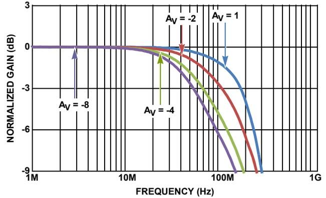
FIGURE 33. INVERTING SMALL SIGNAL RESPONSE vs GAIN
