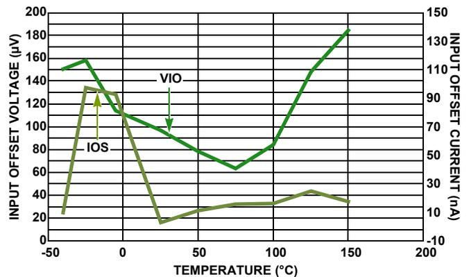
FIGURE 7. INPUT OFFSET VOLTAGE AND CURRENT vs TEMPERATURE
