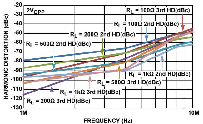
FIGURE 13. INVERTING HD2 AND HD3 vs  $R_{LOAD}$
