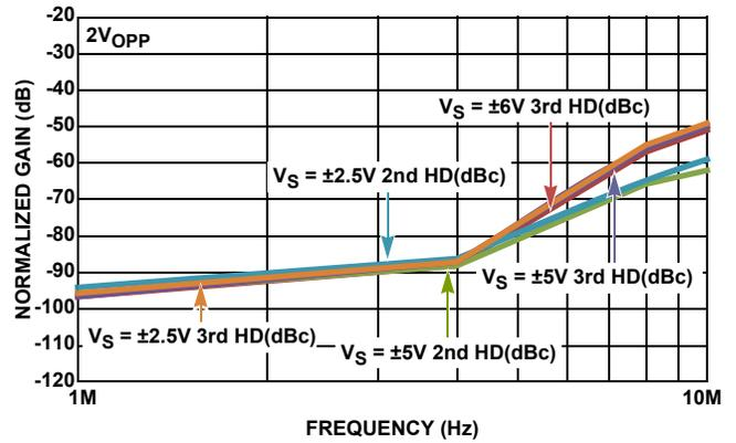
FIGURE 29. INVERTING HD2 AND HD3 vs SUPPLY VOLTAGE
