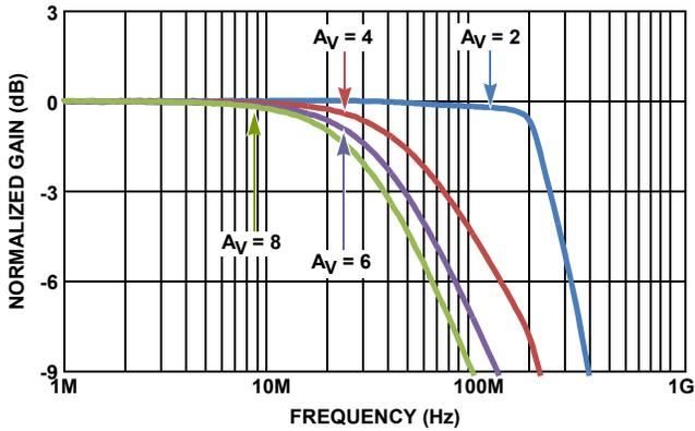
FIGURE 32. NON-INVERTING SMALL SIGNAL RESPONSE vs GAIN
