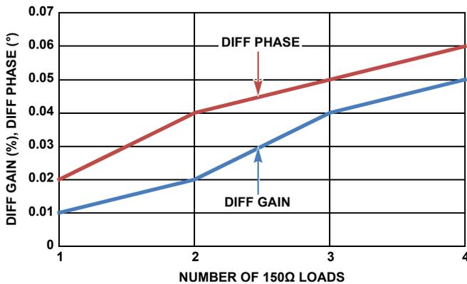
FIGURE 18. DIFFERENTIAL GAIN AND PHASE vs VIDEO LOADS
