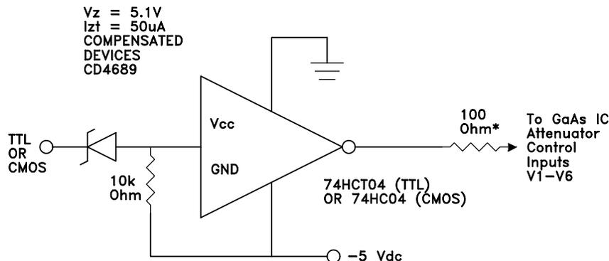
Simple driver using inexpensive standard logic ICs provides fast switching using minimum DC current.
