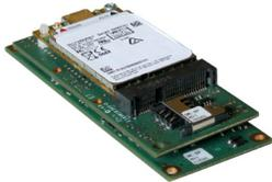
The MultiConnect™ OCG-E embedded open communications gateways with CoreCDP™ comprise an open Linux development environment and a fully certified hardware offering that includes multiple interfaces (serial, USB, Ethernet and SD card) and internal peripherals (including a cellular modem and a GPS receiver) in one application-ready end user solution.
