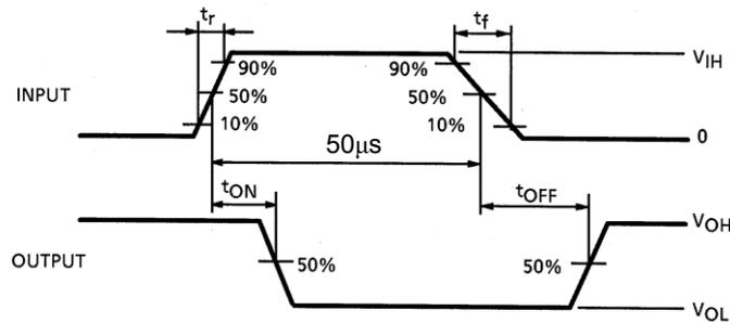
Note 1: Pulse width 50  $\mu$ s, Duty cycle 10%
