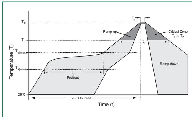
**Flow/Wave Soldering (Solder Dipping)**
