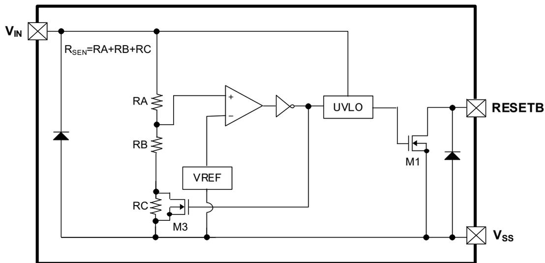
\* Diodes inside the circuits are ESD protection diodes and parasitic diodes
