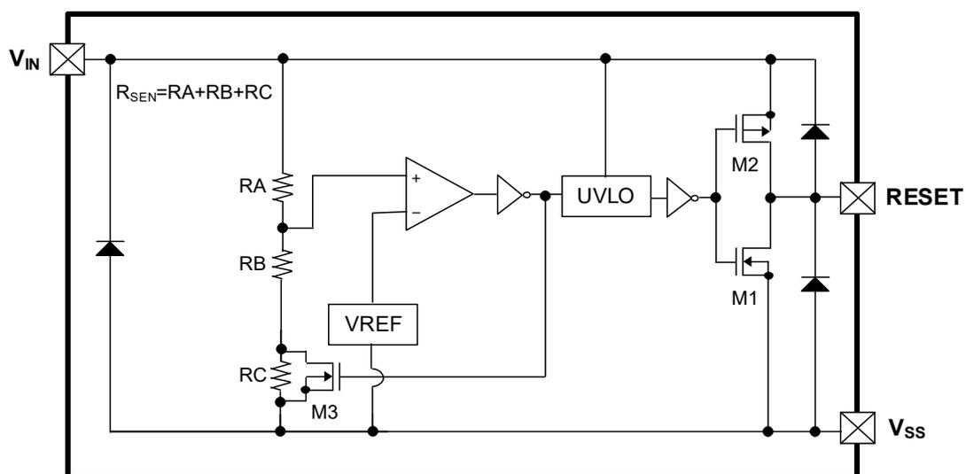
\* Diodes inside the circuits are ESD protection diodes and parasitic diodes.
