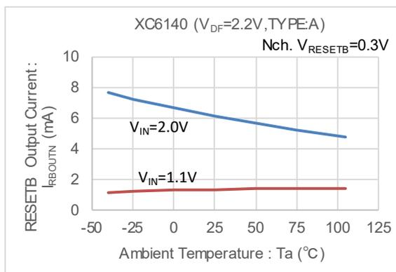
(9) RESETB Output Leakage Current vs. Ambient Temperature
