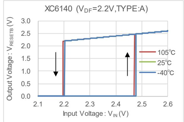
(2) Detect Voltage vs. Ambient Temperature
