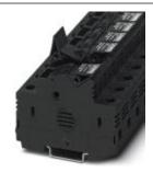
Fuse modular terminal block, Connection method: Screw connection, Cross section: 1.5 mm²- 25 mm², AWG: 16 - 4, Nominal current: 32 A, Nominal voltage: 690 V, Width: 18 mm, Fuse type: Class CC, Fuse type: Glass, Mounting type: NS 35/7,5, NS 35/15, Color: black/red
