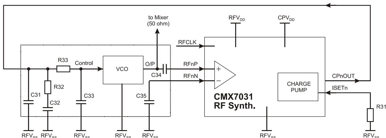
**Figure 14 Example RF Synthesiser Components for a 512MHz Receiver**
