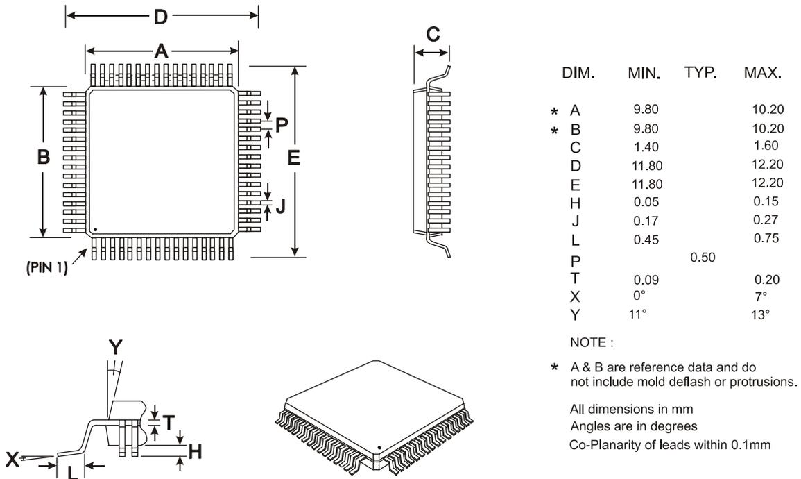
Figure 21 Mechanical outline for 64-pin LQFP (L9)
