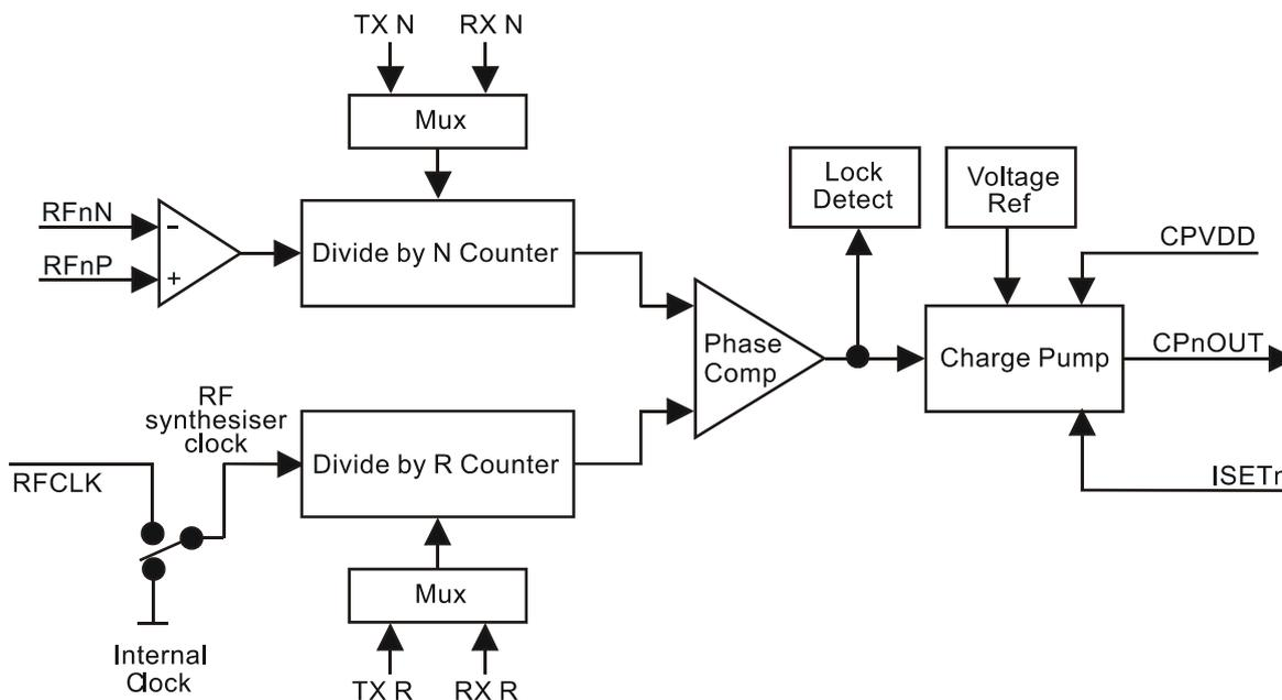
**Figure 15 Single RF Channel Block Diagram**
