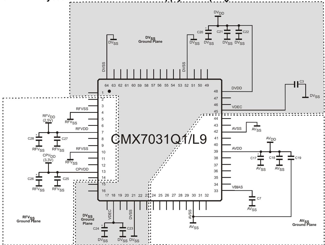
**Figure 4 CMX7031 Power Supply and De-coupling**
