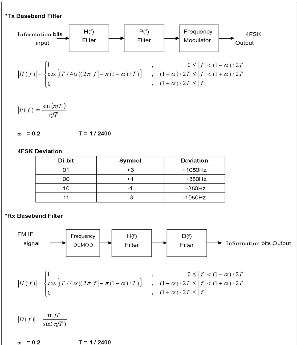
Figure 8 Modulation Characteristics
