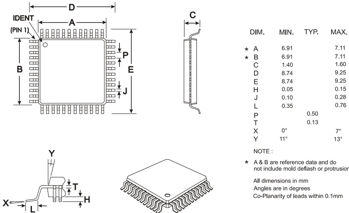
**Figure 23 Mechanical Outline of 48-pin LQFP (L4)**
