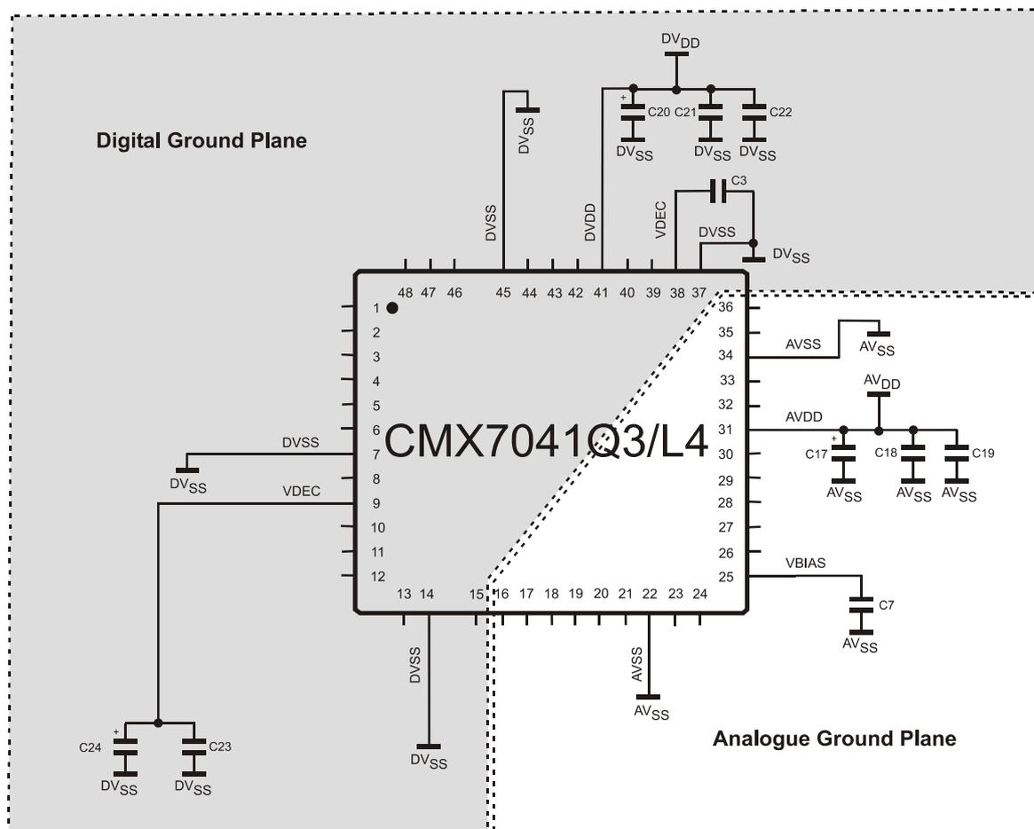
**Figure 5 CMX7041 Power Supply and De-coupling**
