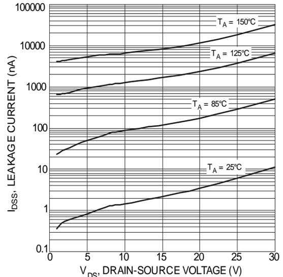
Figure 10 Typical Drain-Source Leakage Current vs. Voltage
