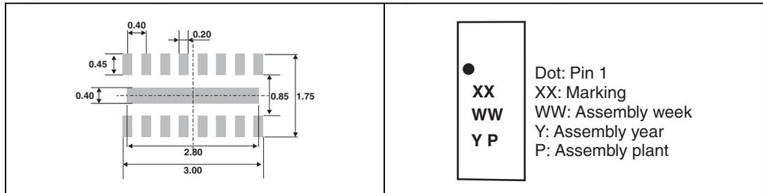
*Note: Product marking may be rotated by 90° for assembly plant differentiation. In no case should this product marking be used to orient the component for its placement on a PCB. Only pin 1 mark is to be used for this purpose.*
