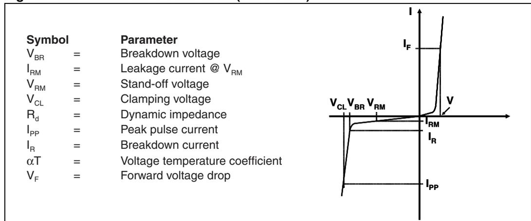
**Table 2. Electrical characteristics ( $T_{amb} = 25\text{ }^{\circ}\text{C}$ )**
