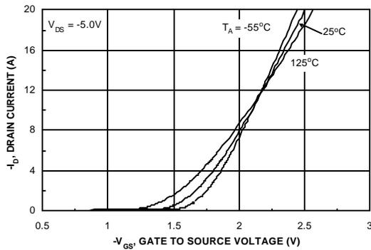
Figure 5. Transfer Characteristics.
