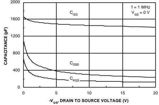
Figure 8. Capacitance Characteristics.
