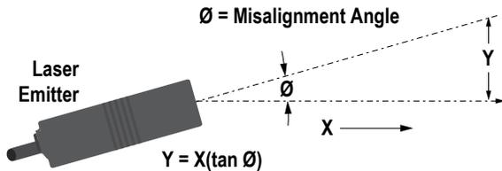
Figure 1. Beam displacement per degree of misalignment
