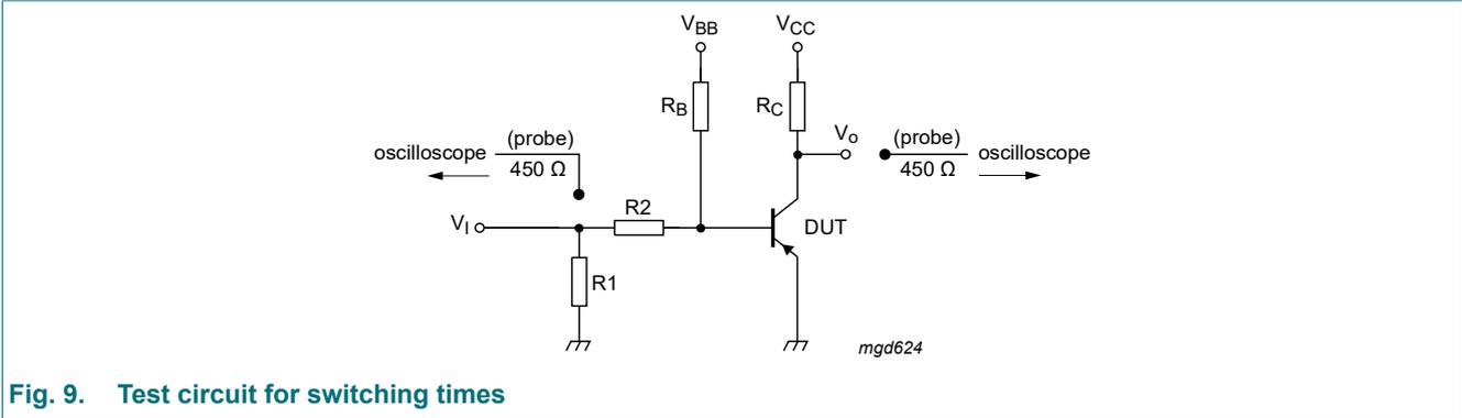
Fig. 9. Test circuit for switching times
