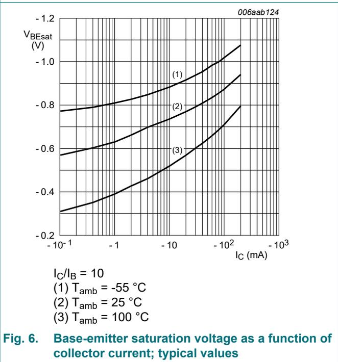
Fig. 6. Base-emitter saturation voltage as a function of collector current; typical values
