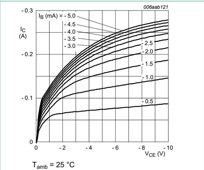
Fig. 4. Collector current as a function of collector-emitter voltage; typical values
