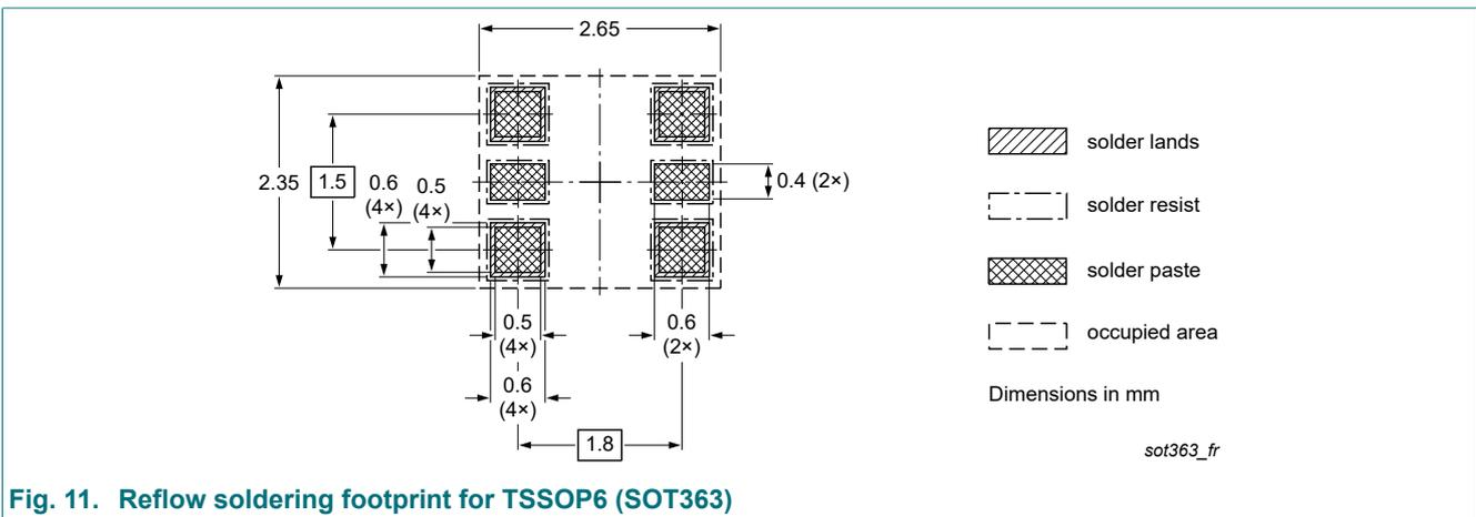
Fig. 11. Reflow soldering footprint for TSSOP6 (SOT363)
