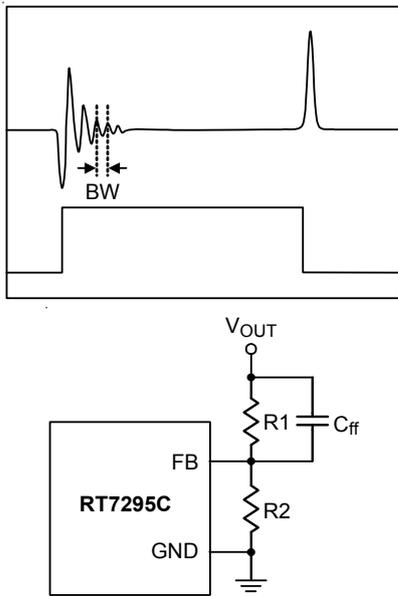
Figure 1. C<sub>ff</sub> Capacitor Setting
