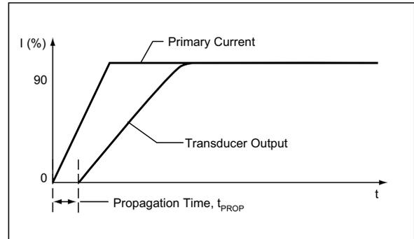
**Response time ( $t_{RESPONSE}$ ).** The time interval between a) when the primary current signal reaches 90% of its final value, and b) when the sensor reaches 90% of its output corresponding to the applied current.
