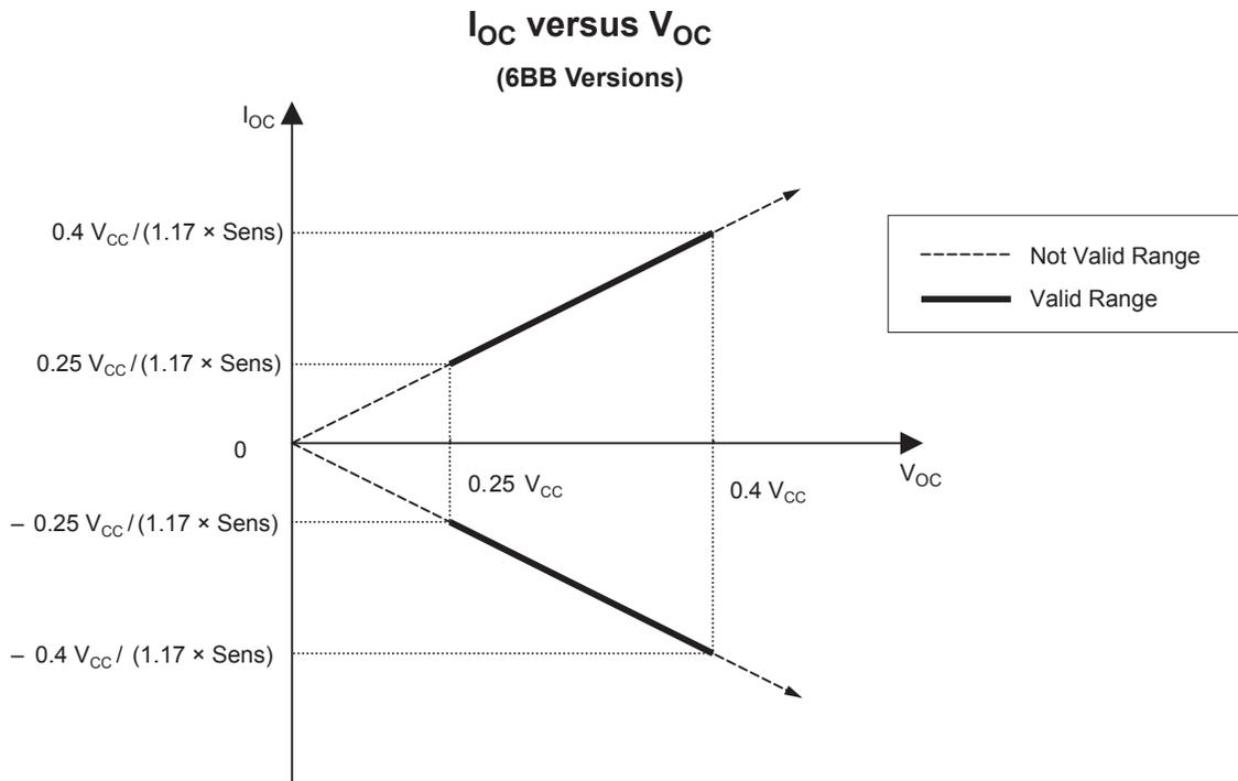
Example: For ACS716KLATR-6BB-T, if required overcurrent fault switchpoint is 10 A, and  $V_{CC} = 3.3$  V, then the required  $V_{OC}$  can be calculated as follows:
