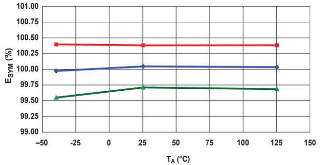
Total Output Error versus Ambient Temperature
