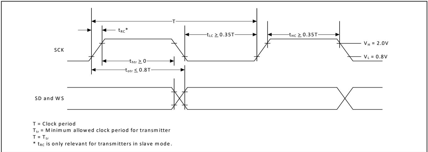
**Figure 17. I<sup>2</sup>S Receiver Timing**
