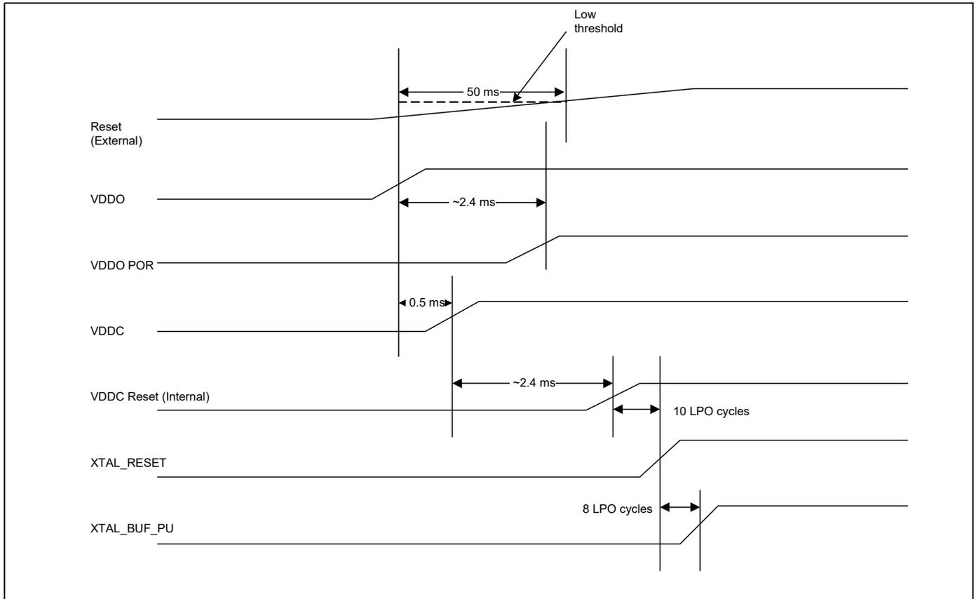
**Note:** The Reset signal should remain below this threshold 50 ms after VDDO is stable. Note that the representation of this signaling diagram is extended and not drawn to scale.
