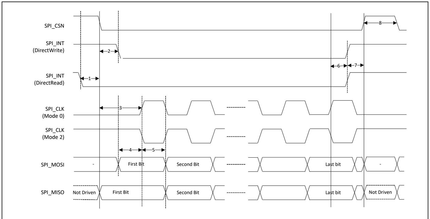
Table 20 and Figure 10 show the timing requirements when operating in SPI Mode 0 and 2.
