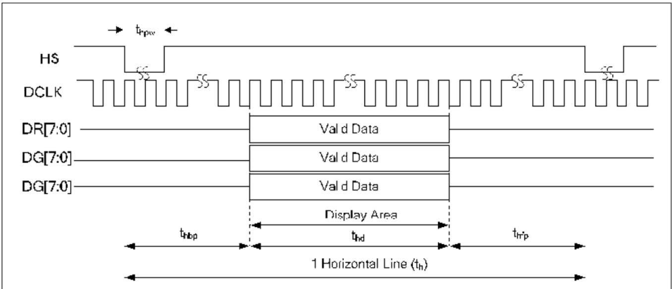
Figure 6.2 Horizontal Input Timing for Sync Mode
