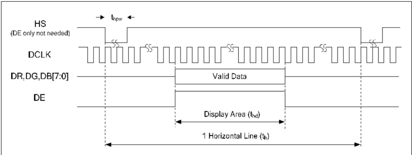
Figure 6.4: Horizontal Input Timing for DE only mode
