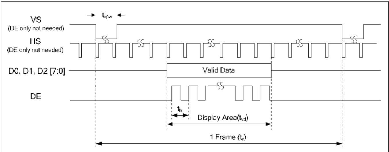
Figure 6.5: Vertical Input Timing for DE only mode
