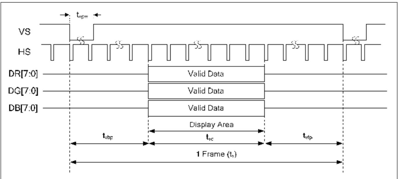
Figure 6.3 Vertical Input Timing for Sync Mode
