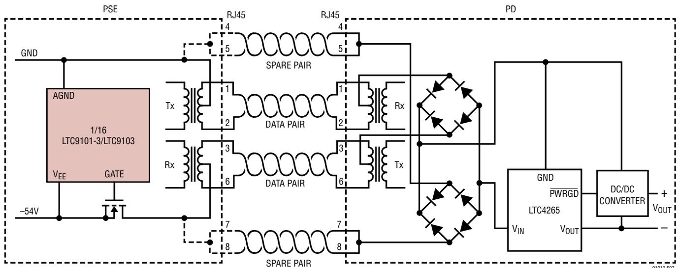
Figure 7. Power Over Ethernet System Diagram, Spare or Data Pairs
