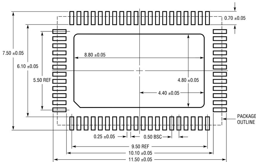
APPLY SOLDER MASK TO AREAS THAT ARE NOT SOLDERED
