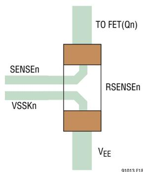
Figure 18. R<sub>SENSE</sub> Kelvin Connections
