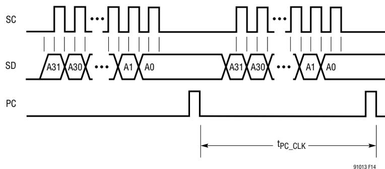
Figure 14. LTC9101-3/LTC9103 SC, SD, and PC Waveform
