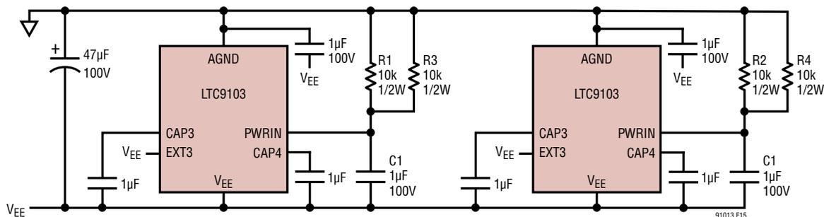
Figure 15. Power Supply Configuration with Internal 3.3V Supply
