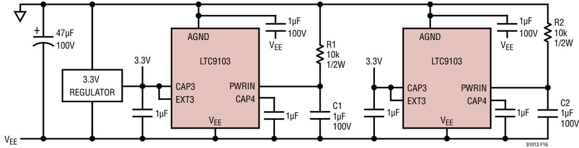
Figure 16. Power Supply Configuration with External 3.3V Regulators
