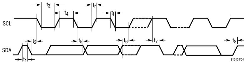
**Figure 4. I<sup>2</sup>C Interface Timing**
