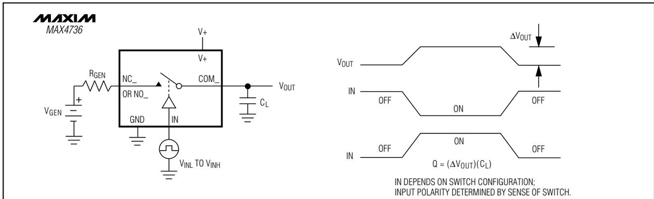
Figure 3. Charge Injection
