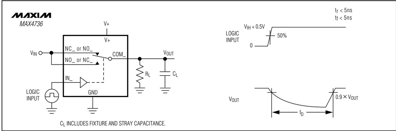
Figure 2. Break-Before-Make Interval
