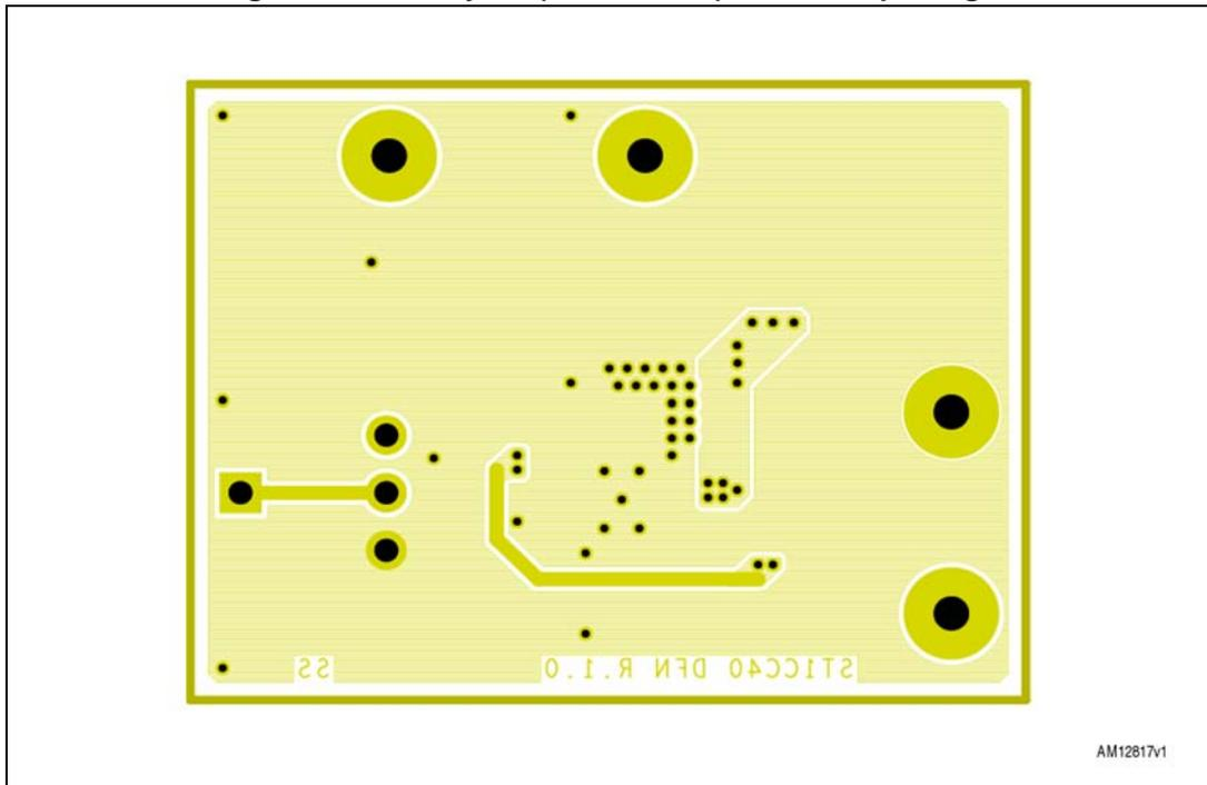
Figure 19. PCB layout (component side) SO8 package
