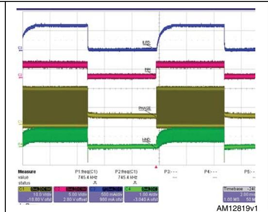
Figure 23. Thermal shutdown protection
