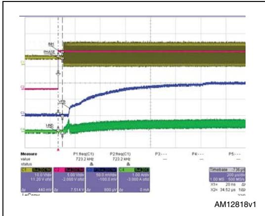
Figure 22. Inhibit operation
