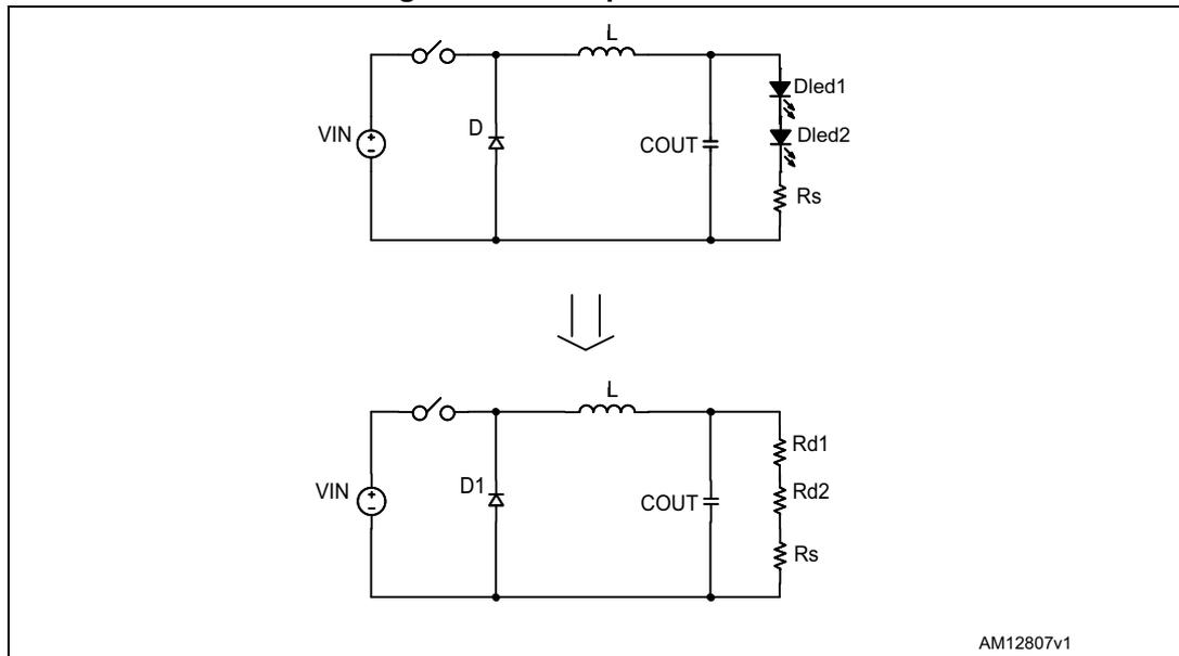
As a consequence, the LED equivalent circuit gives the  $\alpha_{LED}(s)$  term correlating the output voltage with the high impedance FB input:
