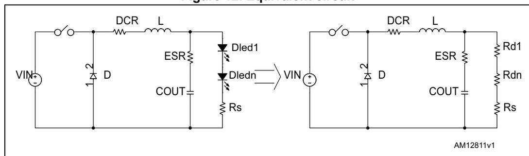
The LED ripple current can be calculated as the inductor ripple current ratio flowing into the output impedance using the Laplace transform (see [Figure 11](#)):
