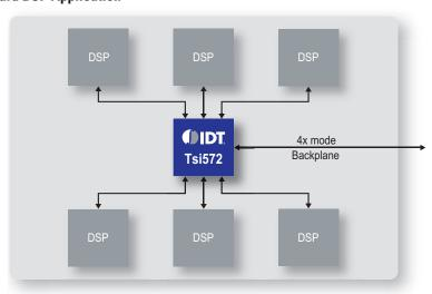
The Tsi572 brings many advantages to wireless applications. It provides a unified platform for WiMAX, eWCDMA, or 3G LTE, and aggregates the key hardware components with three layer hardware termination. It also frees the FPGA, ASIC, DSP and microprocessor resources for application tasks such as OFDMA PHY processing, MAC layer processing, symbol and chip rate processing tasks.
