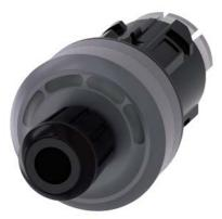
ID key-operated switch, 22 mm, round, plastic with metal front ring, black, RFID, 4 switch positions O-I-II-III, actuating angle 3x45°, without ID key, Z=50-unit packaging
