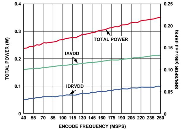
Figure 57. AD9642-250 Power and Current vs. Sample Rate
