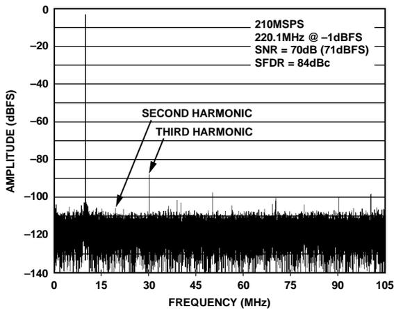
Figure 18. AD9642-210 Single-Tone FFT with  $f_{IN} = 220.1$  MHz
