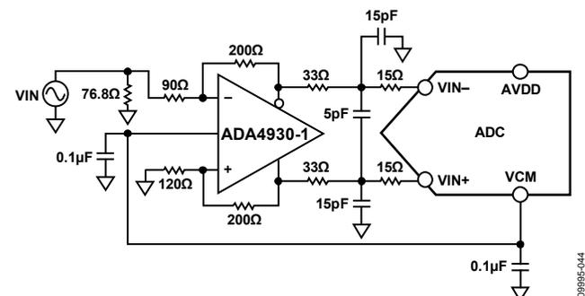
Figure 47. Differential Input Configuration Using the ADA4930-1
