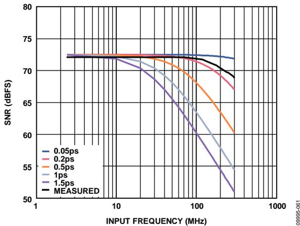
Figure 56. AD9642-250 SNR vs. Input Frequency and Jitter
