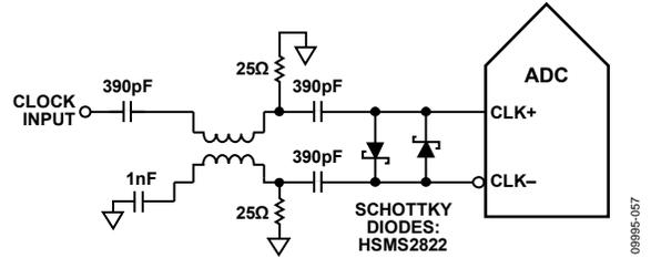
Figure 53. Balun-Coupled Differential Clock (Up to 625 MHz)
