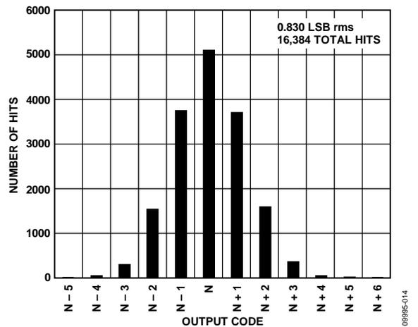
Figure 15. AD9642-170 Grounded Input Histogram,  $f_s = 170$  MSPS
