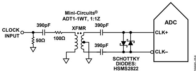
Figure 52. Transformer-Coupled Differential Clock (Up to 200 MHz)
