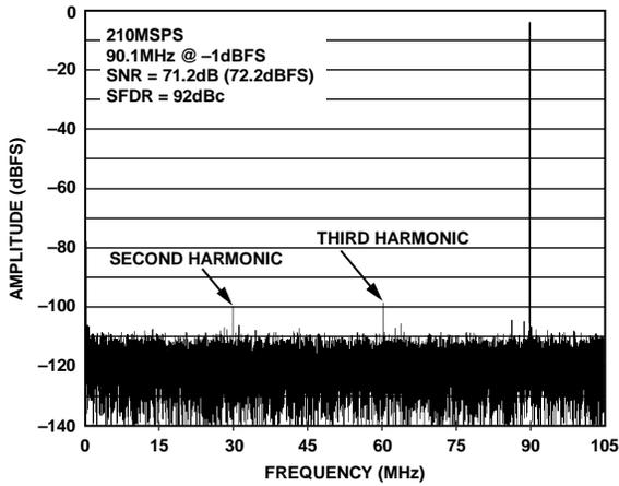
Figure 16. AD9642-210 Single-Tone FFT with  $f_{IN} = 90.1$  MHz
