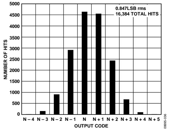
Figure 39. AD9642-250 Grounded Input Histogram,  $f_s = 250$  MSPS
