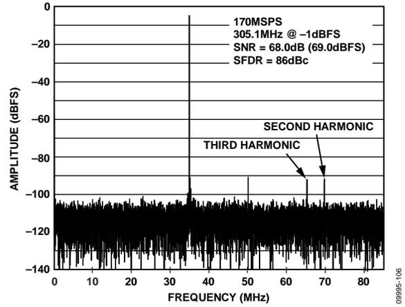
Figure 7. AD9642-170 Single-Tone FFT with  $f_{IN} = 305.1$  MHz
