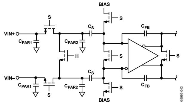
Figure 46. Switched-Capacitor Input
