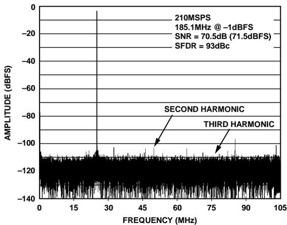
Figure 17. AD9642-210 Single-Tone FFT with  $f_{IN} = 185.1$  MHz
