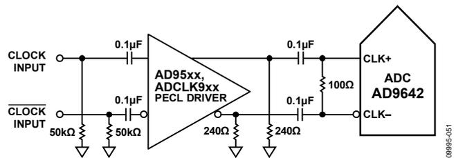
Figure 54. Differential PECL Sample Clock (Up to 625 MHz)
