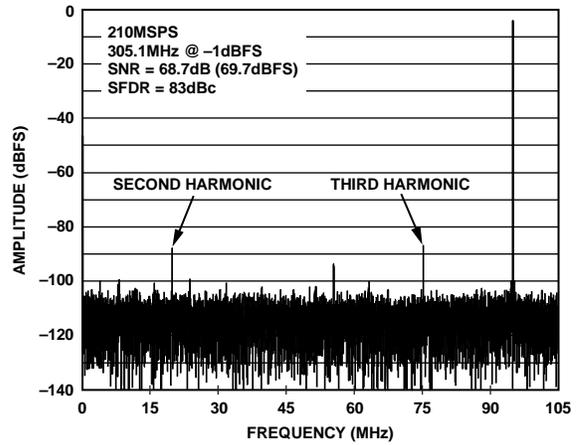
Figure 19. AD9642-210 Single-Tone FFT with  $f_{IN} = 305.1$  MHz
