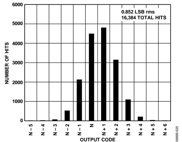
Figure 27. AD9642-210 Grounded Input Histogram,  $f_s = 210$  MSPS
