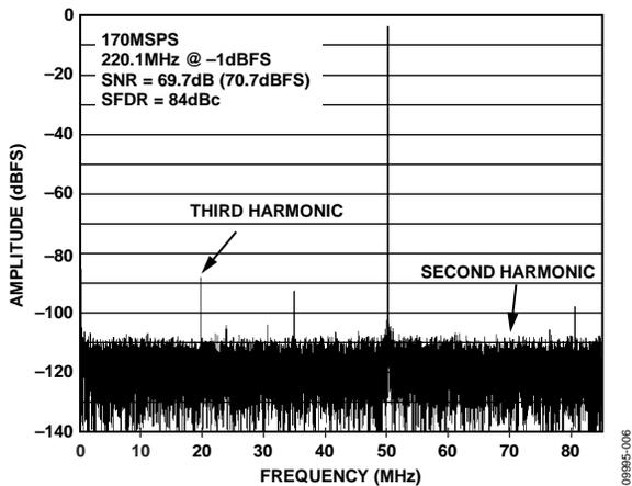
Figure 6. AD9642-170 Single-Tone FFT with  $f_{IN} = 220.1$  MHz
