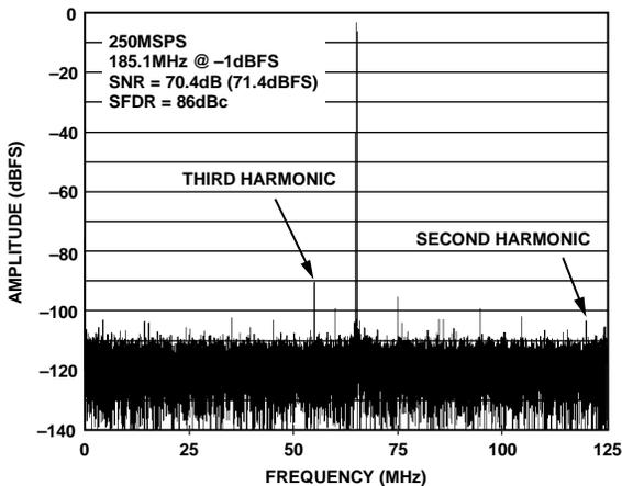
Figure 29. AD9642-250 Single-Tone FFT with  $f_{IN} = 185.1$  MHz
