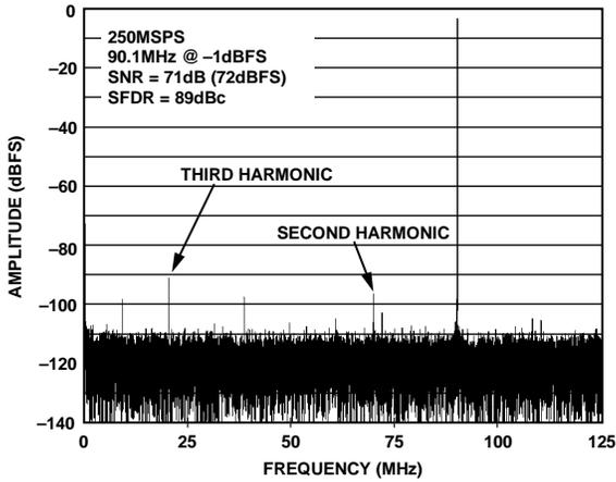
Figure 28. AD9642-250 Single-Tone FFT with  $f_{IN} = 90.1$  MHz
