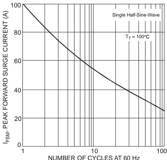
Figure 7 Max Non-Repetitive Peak Forward Surge Current
