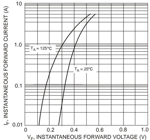
Figure 2 Typical Forward Characteristics – B350BQ/ B360BQ
