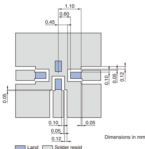
Line width should be designed to match 50Ω characteristic impedance, depending on PCB material and thickness.
