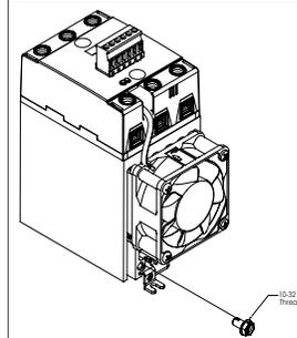
Protective earth (PE) screw type recommended is 10-32 UNC standard not provided with SSR.
