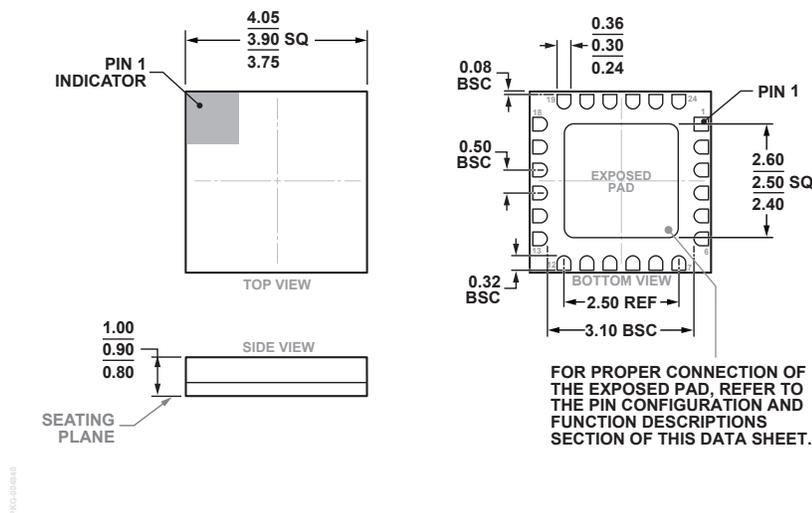
24-Terminal Ceramic Leadless Chip Carrier [LCC]
