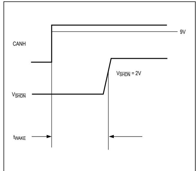
Figure 3. Time to Wake-Up ( $t_{WAKE}$ ) (MAX3050)
