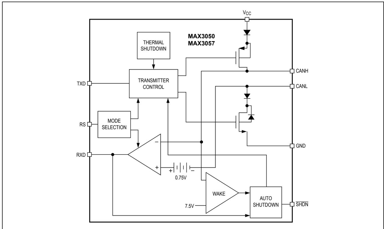
Figure 4. Functional Diagram
