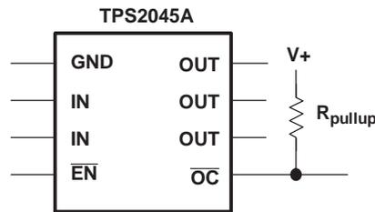
Figure 25. Typical Circuit for  $\overline{OC}$  Pin (Example, TPS2045A)
