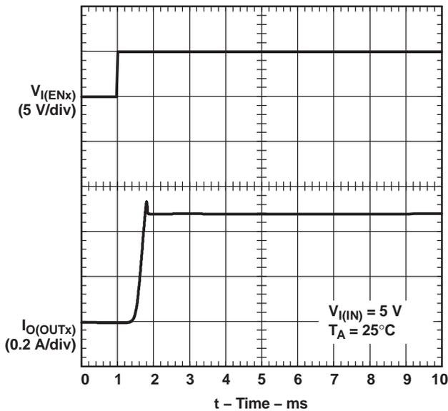
Figure 6. TPS2055A, Short-Circuit Current, Device Enabled Into Short
