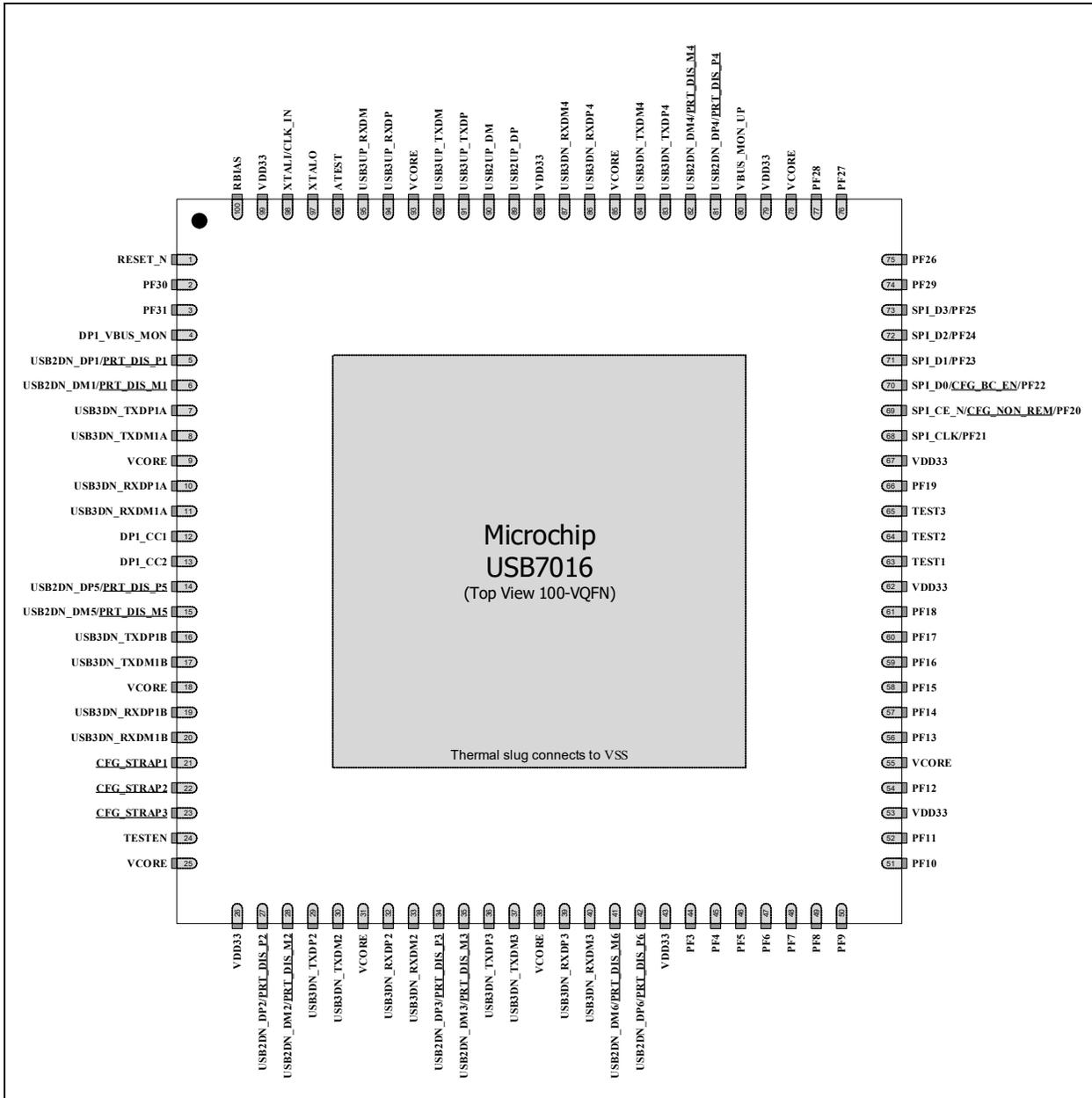
**Note:** Configuration straps are identified by an underlined symbol name. Signals that function as configuration straps must be augmented with an external resistor when connected to a load.
