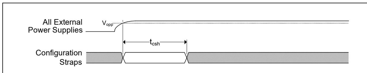
**TABLE 9-5: POWER-ON CONFIGURATION STRAP LATCHING TIMING**
