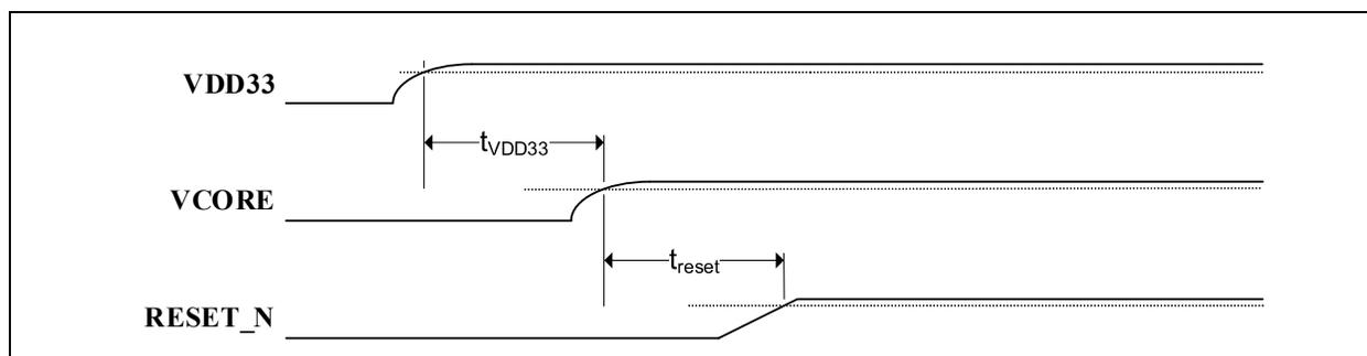
**TABLE 9-4: POWER SUPPLY AND RESET\_N SEQUENCE TIMING**
