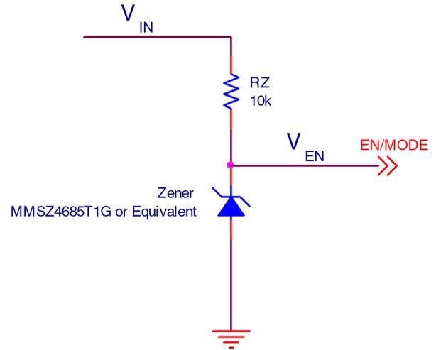
Figure 28: Selecting DCM/CCM by Deriving EN/MODE from  $V_{IN}$
