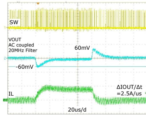
Figure 14: Load Step, Forced CCM, 0A - 7.5 - 0A
