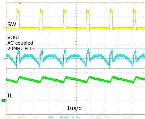
Figure 7:  $V_{OUT}$  Ripple is 14mV at 15A
