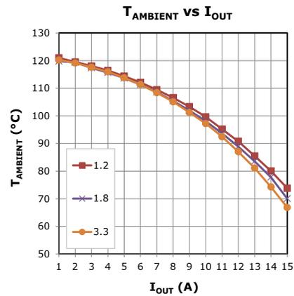
Figure 26: Package Thermal Derating, 5VIN
