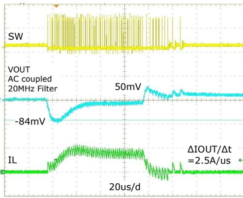
Figure 13: Load Step, DCM / CCM, 0A - 7.5A - 0A
