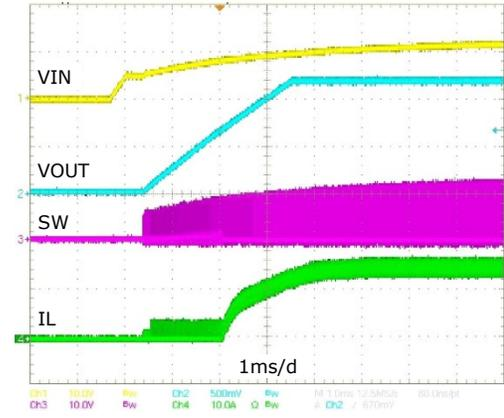
Figure 20: Power-up, DCM / CCM,  $I_{OUT} = 15A$
