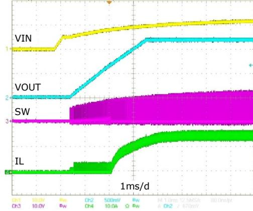
Figure 18: Power-up, Forced CCM,  $I_{OUT} = 15A$
