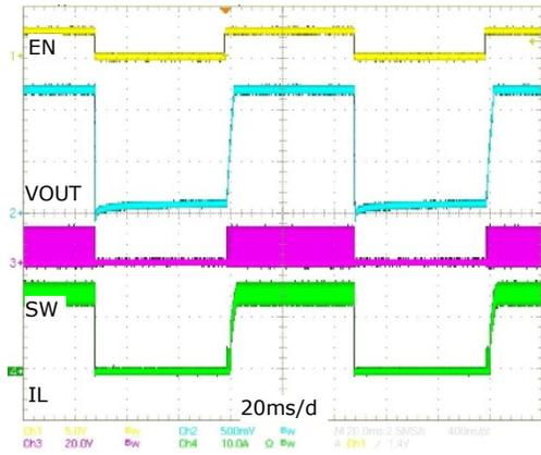
Figure 21: Enable Turn On / Turn Off,  $1.2V_{OUT}$ ,  $15A$
