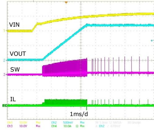
Figure 19: Power-up, DCM / CCM,  $I_{OUT} = 0A$
