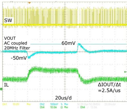
Figure 15: Load Step, Forced CCM, 7.5A - 15A - 7.5A
