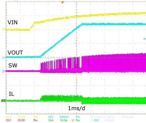
Figure 17: Power-up, Forced CCM,  $I_{OUT} = 0A$
