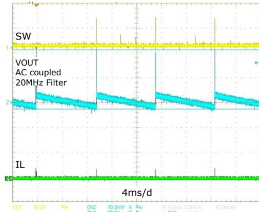
Figure 8:  $V_{OUT}$  Ripple is 23mV at 0A, DCM
