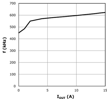
Figure 9: Frequency vs.  $I_{OUT}$ , Forced CCM
