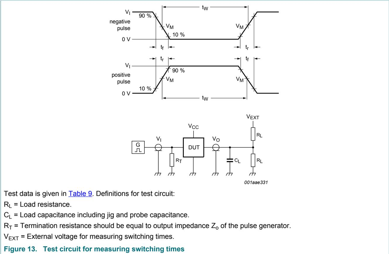
Test data is given in [Table 9](#). Definitions for test circuit:
