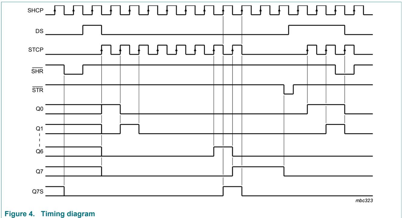
Figure 4. Timing diagram
