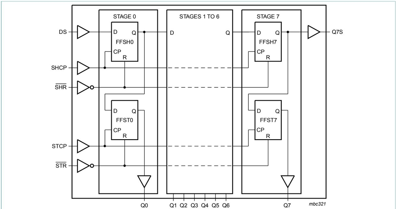
Figure 3. Logic diagram
