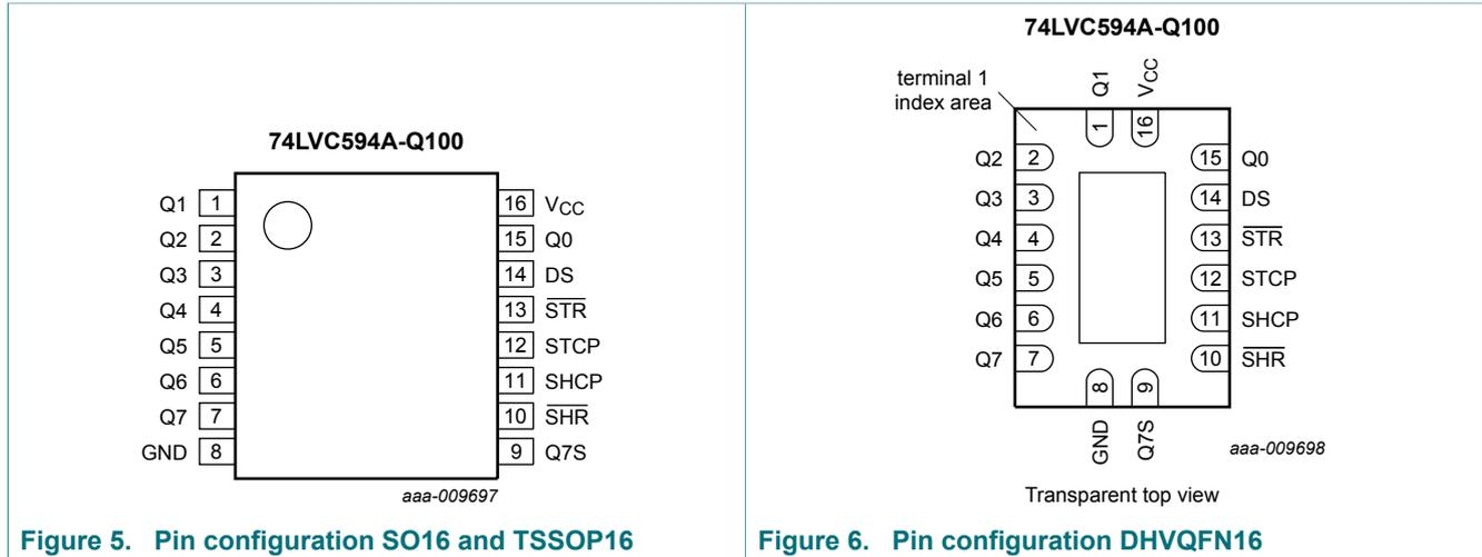
Figure 5. Pin configuration SO16 and TSSOP16
