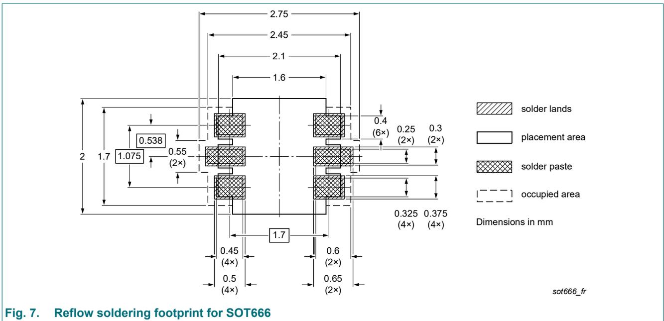
Fig. 7. Reflow soldering footprint for SOT666
