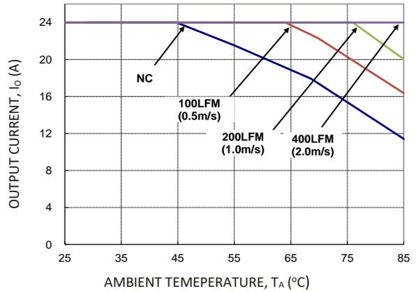
**Figure 20. Output Current Derating for the Module with 18 Heatplate; Airflow in the Transverse Direction from V<sub>out</sub>(-) to V<sub>out</sub>(+); V<sub>IN</sub>=24V, V<sub>O</sub>=5V.**
