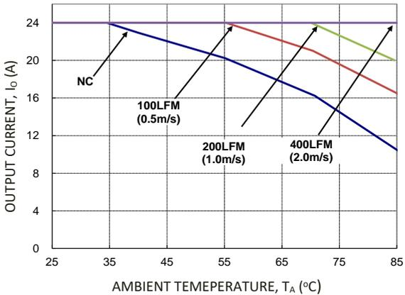
**Figure 18. Output Current Derating for the Open Frame Module; Airflow in the Transverse Direction from V<sub>out</sub>(-) to V<sub>out</sub>(+); V<sub>IN</sub>=24V, V<sub>O</sub>=5V.**
