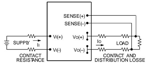
Figure 11. Circuit Configuration for remote sense .
