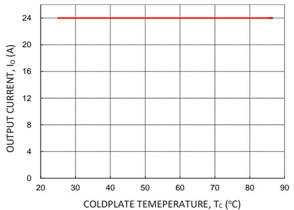
**Figure 22. Derated Output Current versus Cold Wall Temperature with local ambient temperature around module at 85C; V<sub>IN</sub>=24V or 48V.**
