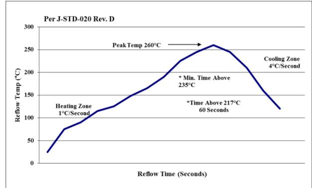
**Figure 26. Recommended linear reflow profile using Sn/Ag/Cu solder.**
