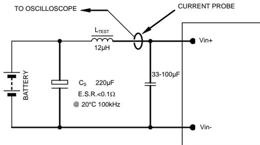
NOTE: Measure input reflected ripple current with a simulated source inductance ( $L_{TEST}$ ) of 12µH. Capacitor  $C_S$  offsets possible battery impedance. Measure current as shown above.
