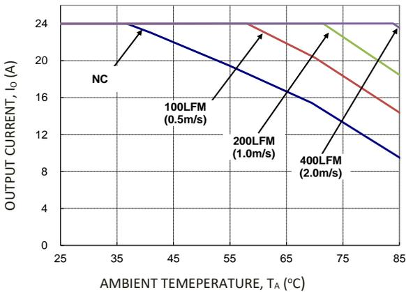
**Figure 19. Output Current Derating for the Module with Heatplate; Airflow in the Transverse Direction from V<sub>out</sub>(-) to V<sub>out</sub>(+); V<sub>IN</sub>=24V, V<sub>O</sub>=5V.**
