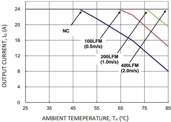
**Figure 17. Output Current Derating for the Module with 18H Heatplate; Airflow in the Transverse Direction from V<sub>out</sub>(-) to V<sub>out</sub>(+); V<sub>IN</sub>=48V, V<sub>O</sub>=5V**
