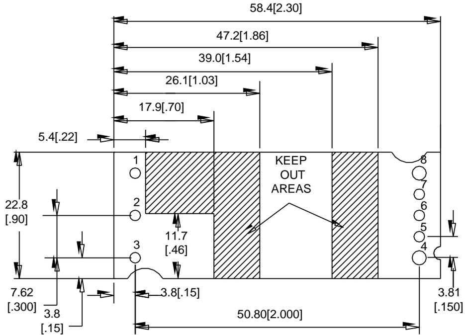
**SMT Recommended Pad Layout (Component Side View)**
